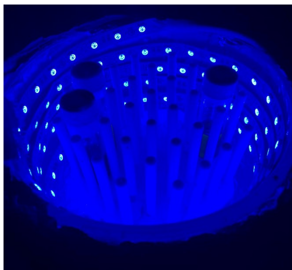
Figure S1. Reaction setup for the photoinduced formation of chloroalkanes
