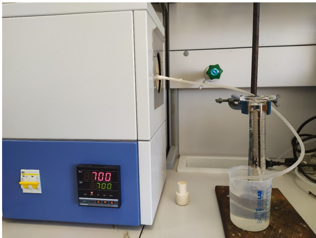
Figure S1. Hydrogen generation experiment system
