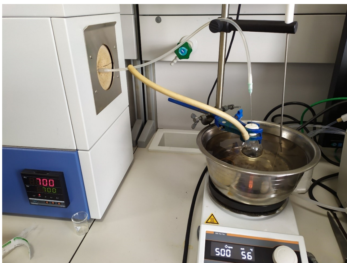
Figure S2. Hydrogenation using hydrogen from CCRs
