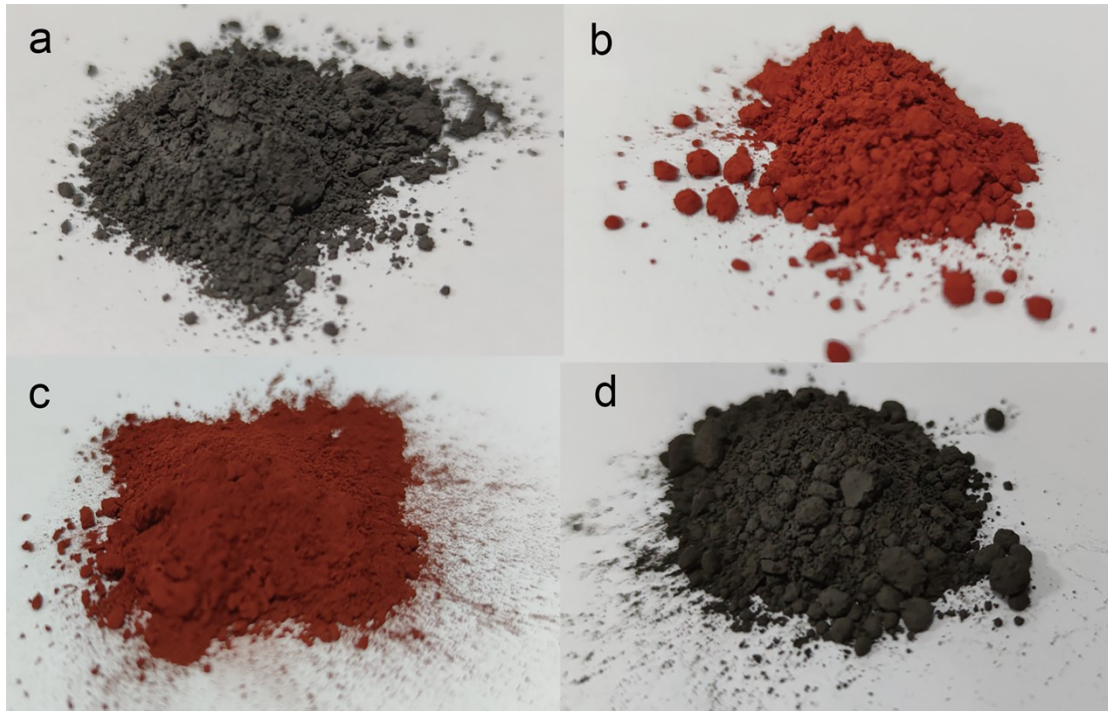
Fig. S1. Photograph of (a) spent, (b) homogenized, (c) spray-dried and (d) regenerated \text{LiFePO}_4
