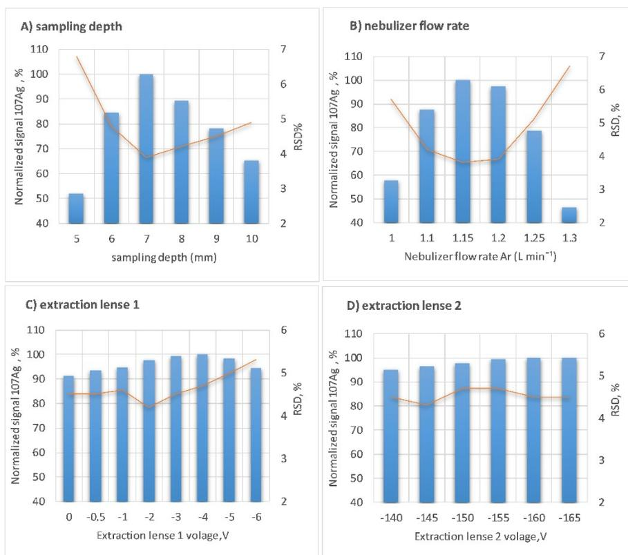
Figure S2.1 Influence of instrumental parameters on the sensitivity and stability of signals for  $^{107}\text{Ag}$ . The red line indicates the RSD value in % on second axis. Constant values during optimization are: A) nebulizer gas flow rate –  $1.2\ \text{L min}^{-1}$ . B), sampling depth - 7 mm, C) and D) sampling depth 7, nebulizer flow rate 1.15
