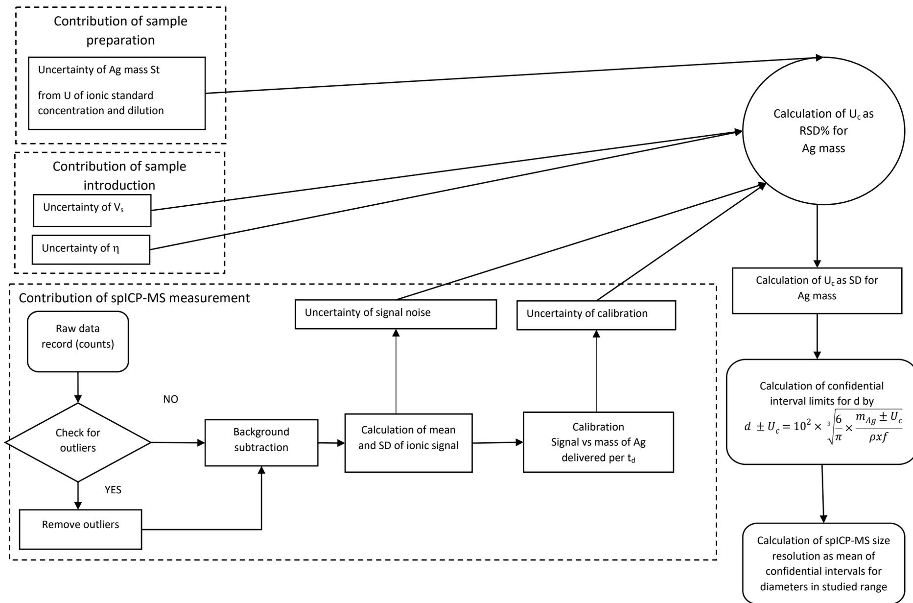
Figure S2.2 A flow-chart diagram for NPs size uncertainty estimation and spICP-MS size resolution determination using ionic standard calibration approach.
