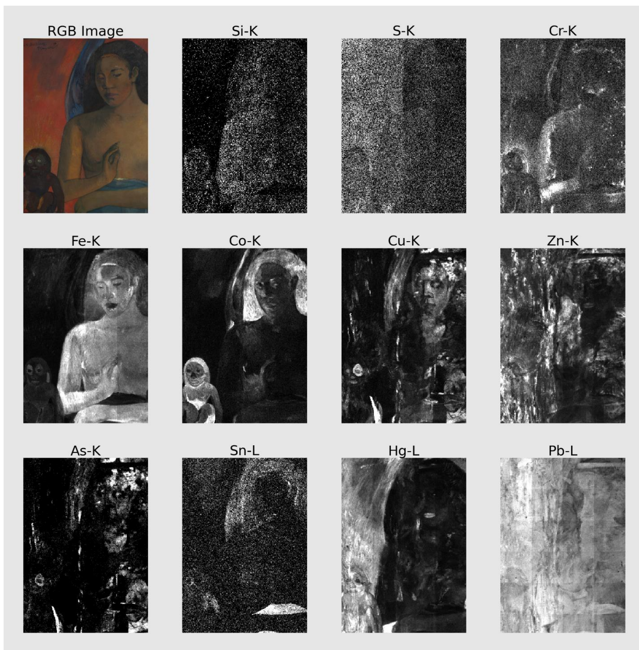
Figure S1. Elemental maps of the Gauguin painting obtained using PyMCA. Elements identified include silicon (Si), sulfur (S), chromium (Cr), iron (Fe), cobalt (Co), copper (Cu), zinc (Zn), arsenic (As), tin (Sn), mercury (Hg) and lead (Pb).
