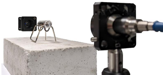
Figure S 8. Image of the quartz tube used in the additional FAA setup. The illumination light was fed through a 600- \mu\text{m} diameter optical fiber and a collimator (F810SMA-543, Thorlabs). The collection optics was placed at the downstream of the optical path after the quartz sampling chamber. The beam was then refocused at the collector with a plano-convex lens ( f = 50 \text{ mm} LA1131, Thorlabs). The collected light was directed to the spectrometer through another 600- \mu\text{m} optical fiber.
