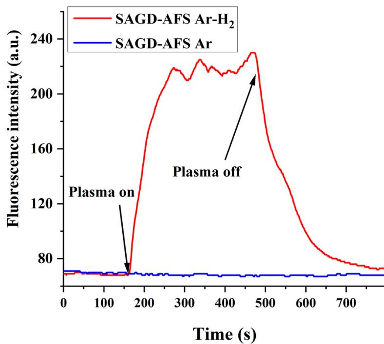
Figure S1. Fluorescence spectra of As detected by SAGD-AFS under Ar and Ar-H<sub>2</sub> atmosphere.
