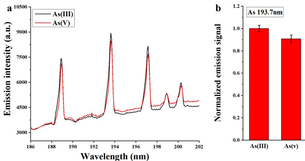
Figure S3. a) The emission spectra and b) the comparison of normalized emission signal normalized signal in 193.7 nm of As (III) and As(V) by hydrogen-doped SAGD-OES.
