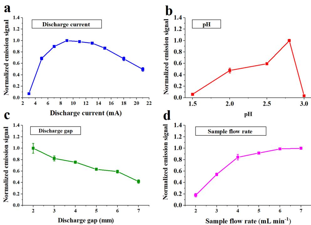
Figure S4. Optimization of the SAGD-OES parameters: the effect of a) discharge current, b) pH, c) discharge gap and d) sample flow rate on As emission signal (Ar flow rate: 300 mL min<sup>-1</sup>; H<sub>2</sub> flow rate: 15 mL min<sup>-1</sup>.)
