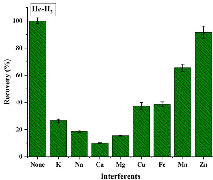
Figure S6. The effect of concomitant ions (10 mg L<sup>-1</sup>) on recovery of As detected by He-H<sub>2</sub> SAGD-OES.
