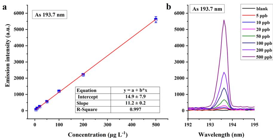
Figure S5. a) The standard curve and b) emission spectra of As at different concentrations.
