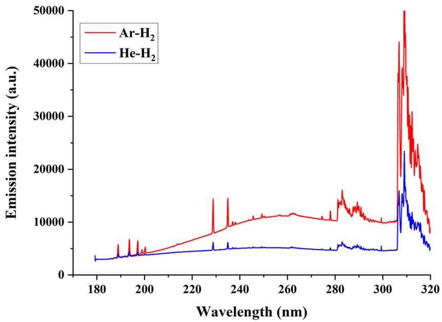
Figure S2. The emission spectra of As under Ar-H<sub>2</sub> and He-H<sub>2</sub> (including the background spectra).
