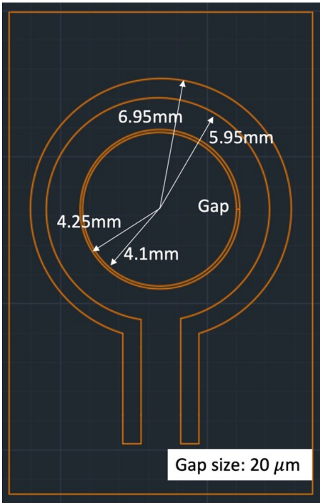
Figure S2. Microwave sensor structure and dimensions
