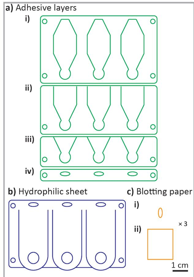
Figure 1: Layout of three microfluidic chambers indicating: **a) i), ii), iii), iv)** the adhesive layers; **b)** the hydrophilic sheet; **c) i), ii)** the blotting papers.
