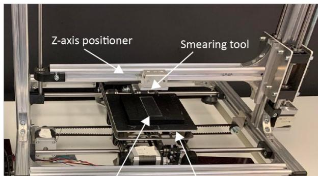
Figure 3: Picture of the robotic stage displaying the smearing tool attached to the Z-axis positioner and the glass slide on top of the XY-axis platform.
