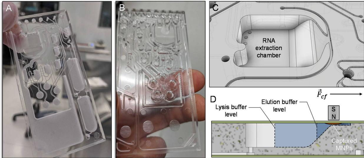
**Fig. S1** Microfluidic cartridge. (A) Photograph showing a cartridge variant that was fabricated using CNC machining. (B) Center piece produced by injection molding. (C) 3D design representation of the RNA extraction chamber. (D) Cross-section schematic showing the profile of the RNA extraction chamber, liquid levels for lysis buffer and elution buffer, as well as position of the MNPs after capture with the magnet. The direction of flow is from left to right.
