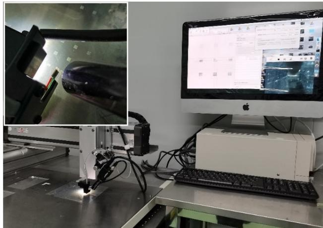
**Figure S1.** The equipment for the PC-FLISA (photonic crystal-fluorescence immunosorbent assay) biochip. The inset is an enlarged picture of the printing chip.
