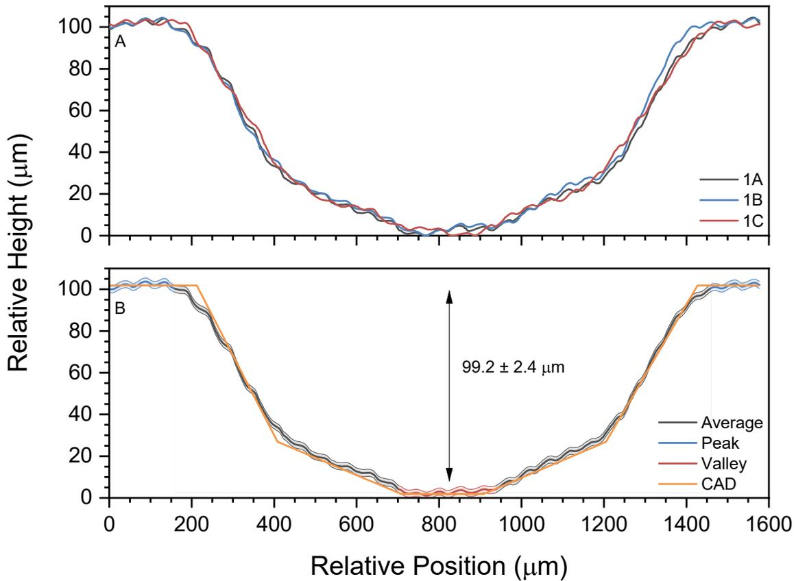
Fig. S2. Profilometry of series 1 stripping half-modules. These half-modules were printed together at the same time. (A) Profile of each half-module translated on top of each other. (B) Average profile with the peaks in blue and the valley in red. The geometry of the CAD drawing of the channel is in gold. The shaded area in (B) represents the average surface variation around the mean.
