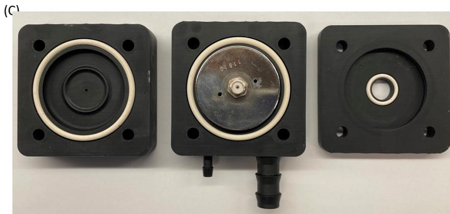
Fig. S4. Alpha chamber design. The CAD schematic (A) is shown with o-ring grooves and bolt clearance holes omitted for clarity. The distance between the sample and detector surface is
