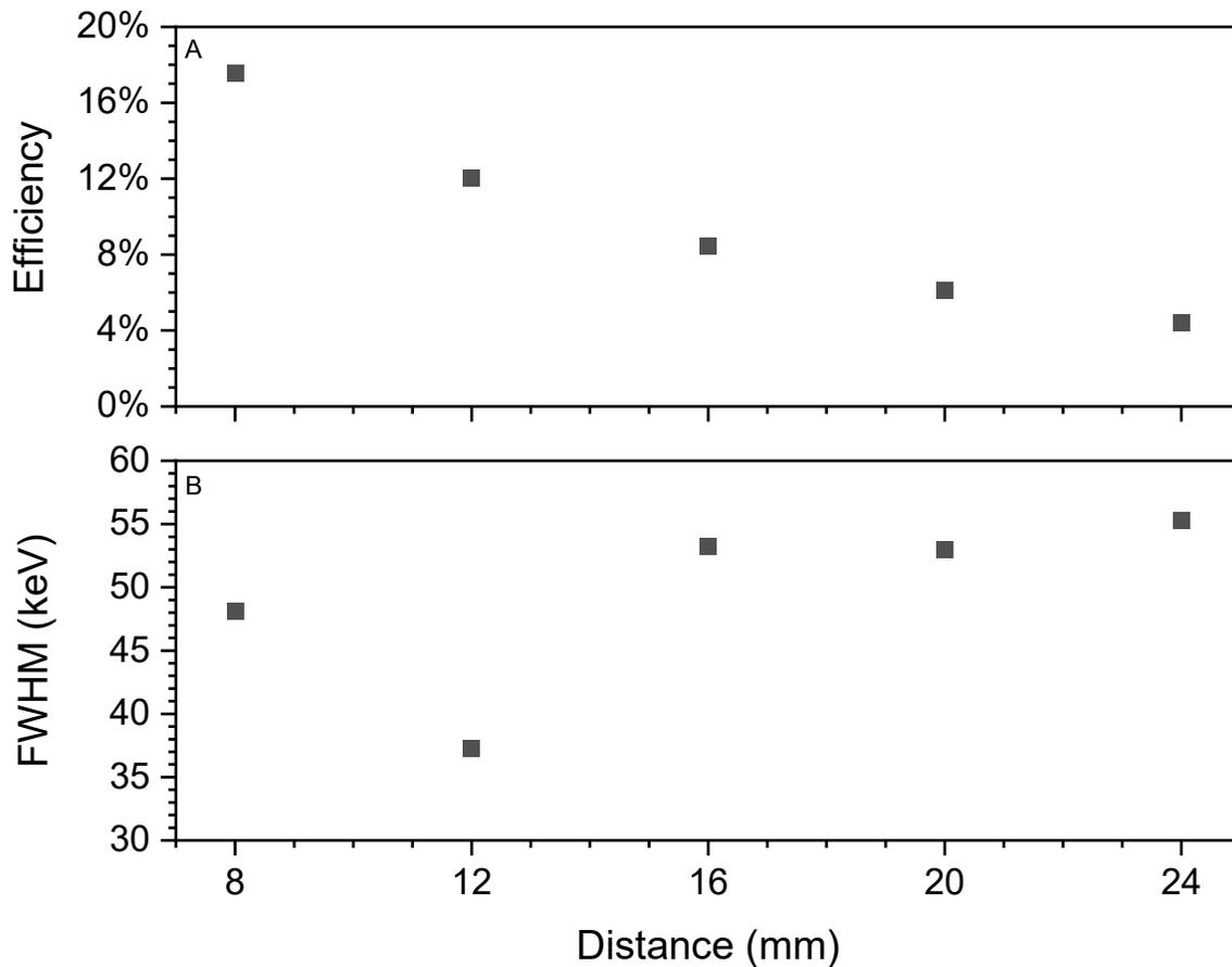
Fig. S5. Characteristics of the 3D alpha chamber. (A) Efficiency and (B)  $^{238}\text{Pu}$  peak FWHM as a function of detector distance from sample stage.
