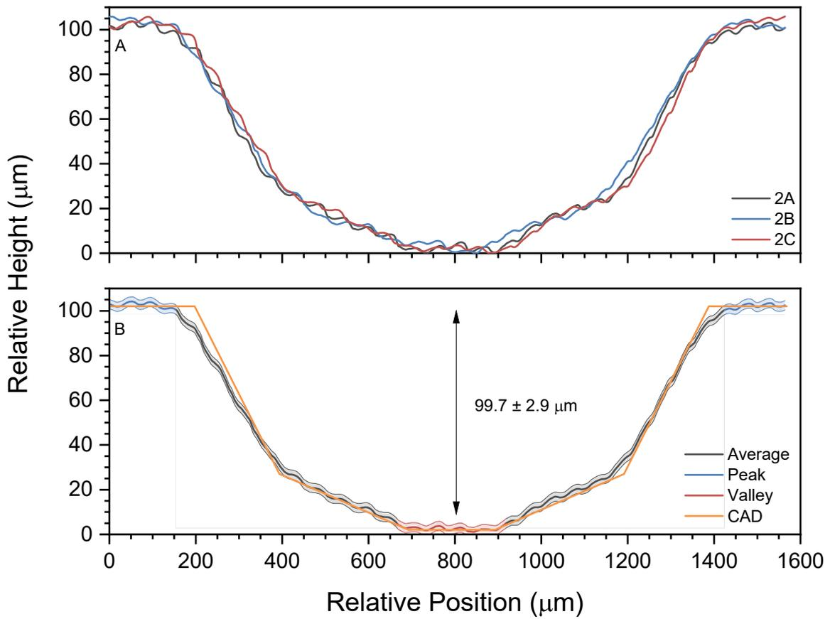
Fig. S3. Profilometry of series 2 stripping half-modules. These half-modules were printed two weeks after series 1. (A) Profile of each half-module translated on top of each other. (B) Average profile with the peaks in blue and the valley in red. The geometry of the CAD drawing of the channel is in gold. The shaded area in (B) represents the average surface variation around the mean.
