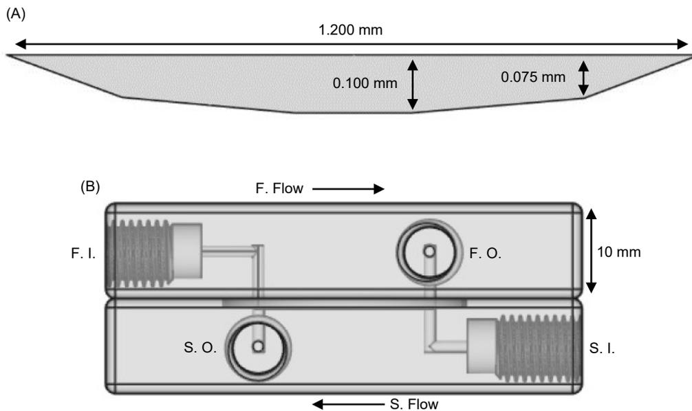
Fig. S1. FS-SLM design and production. (A) Dimensions of the 6-sided irregular polygon cross-section used for the 192 mm extraction channel. (B) Schematic view of an assembled
