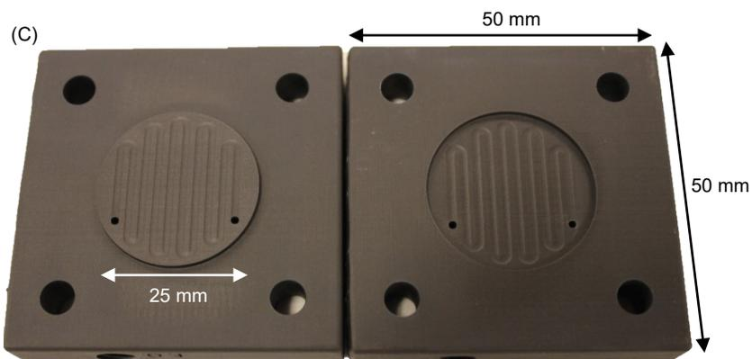
FS-SLM module with counter-current flow where F refers to the feed stream, S the stripping stream, I an inlet, and O an outlet. (C) Picture of a 3D printed feed (left) and stripping (right)
