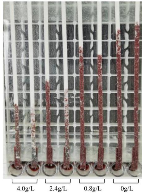
**Figure S5.** Comparison of the wicking length of the whole blood samples of four different fibrinogen concentrations on test strips. It can be seen from the figure that the fibrinogen concentrations have significant influence on the wicking lengths.
