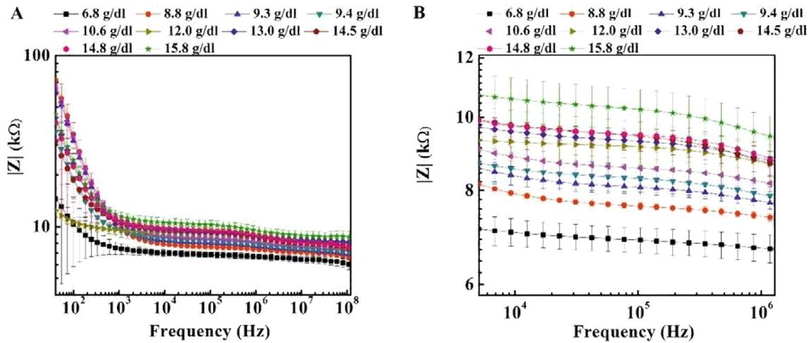
**Fig. S4.** (A) The impedance spectra of whole blood samples having different Hb values (g/dl) swept over the entire frequency spectrum between 40 Hz to 110 MHz, (B) Impedance spectra between 50 kHz to 1MHz frequency range for the blood samples.
