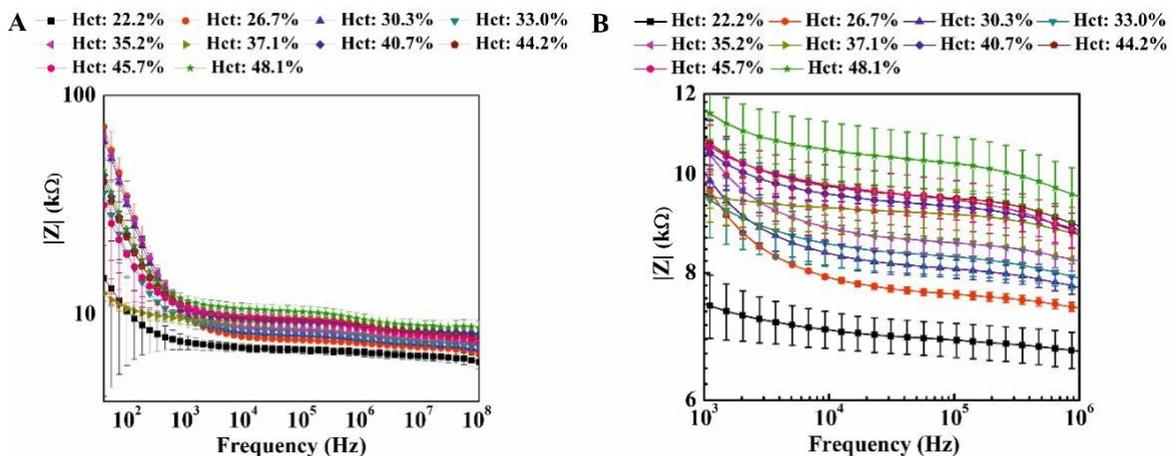
**Fig. S3.** (A) The impedance spectra of whole blood samples having different Hct (%) swept over the entire frequency spectrum between 40 Hz to 110 MHz, (B) Impedance spectra between 10 kHz to 1MHz frequency range for the blood samples.
