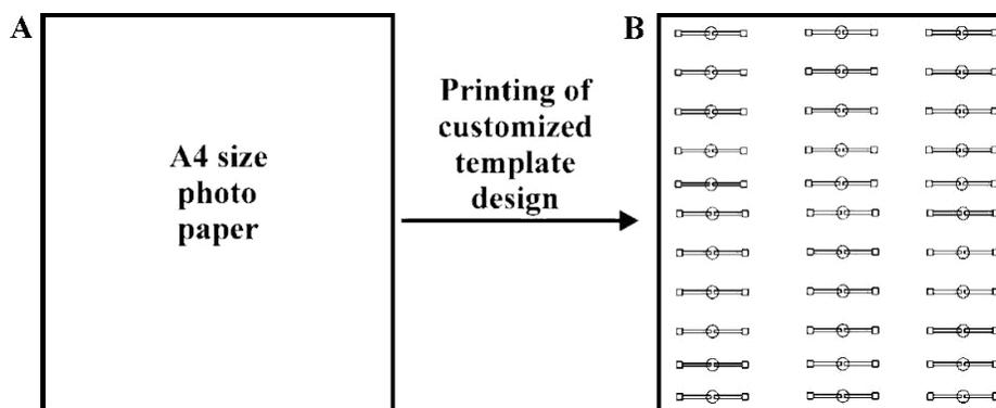
**Fig. S1.** Schematic of the sensor template mass fabrication (A) Substrate: A4 size photo paper. (B) The sensor array is printed on the non-glossy side of the photo paper.
