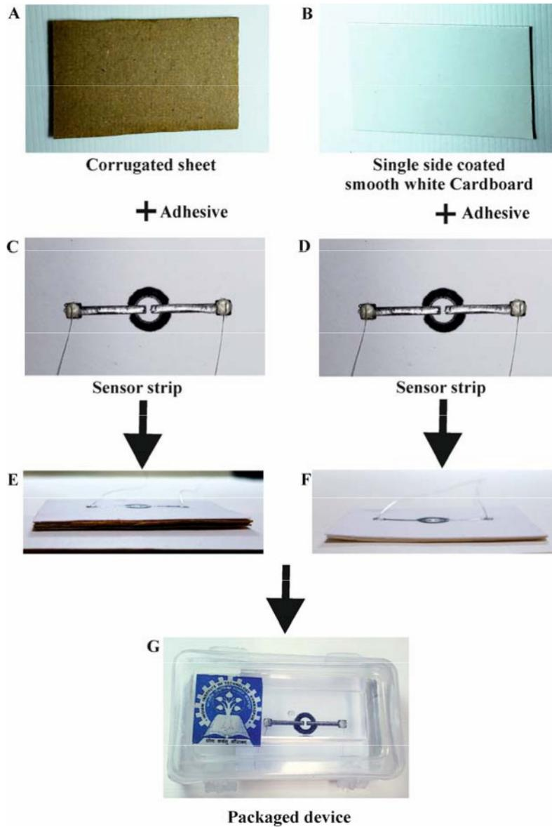
**Fig. S6.** Packaging and storage of device (A) Corrugated sheet (B) Single side coated smooth white cardboard (C) & (D) Disposable paper and pencil sensor strip (E) & (F) Side view of the device adhered to the corrugated sheet and single side coated smooth white cardboard, respectively, (G) Final packaged device inside transparent plastic box for long term storage. .
