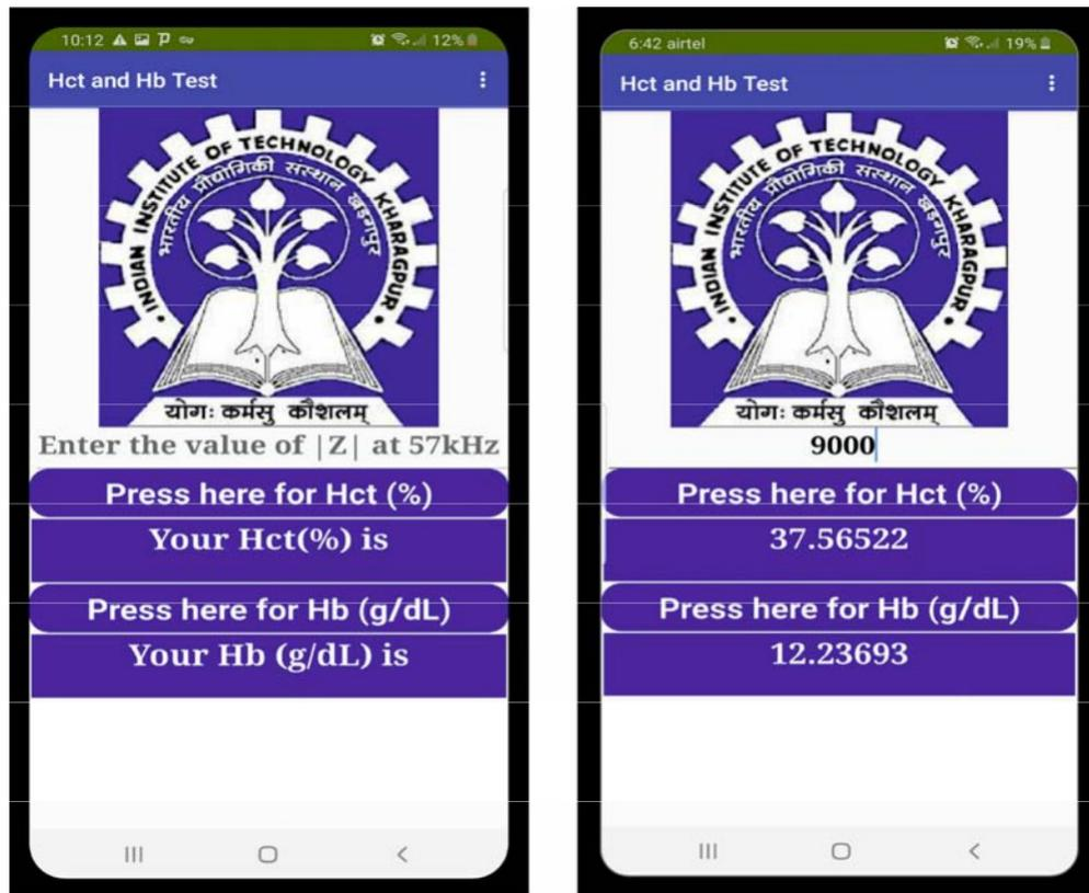
**Fig. S5.** Graphical user interface of the in-house developed Hct and Hb Test app for user-friendly Hct and Hb level determination based on the calibration code.
