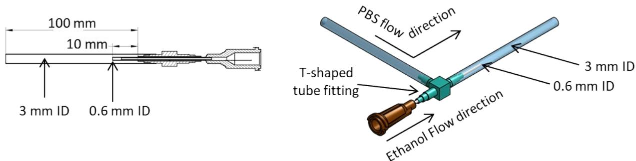
*Figure S1. Schematic view of the fabricated coaxial millifluidic mixer.*
