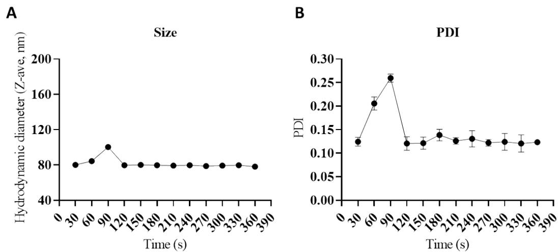
**Figure S7. Stability of the liposome size (A) and PDI (B) after running the setup for 360 seconds.**
