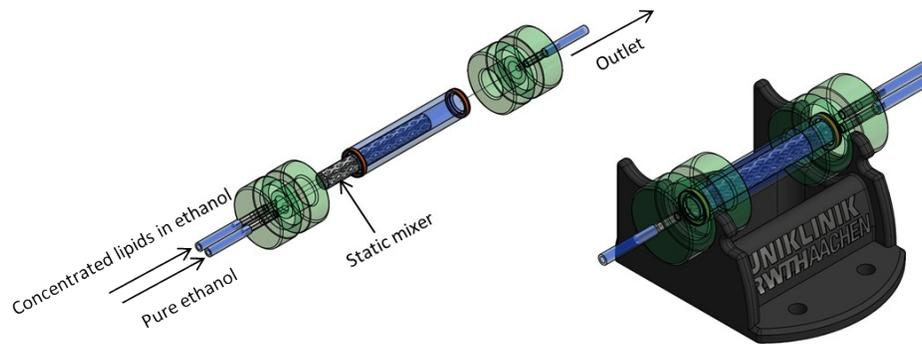
Figure S3. Schematic view of the static mixer for proper mixing of the concentrated lipids and pure ethanol.
