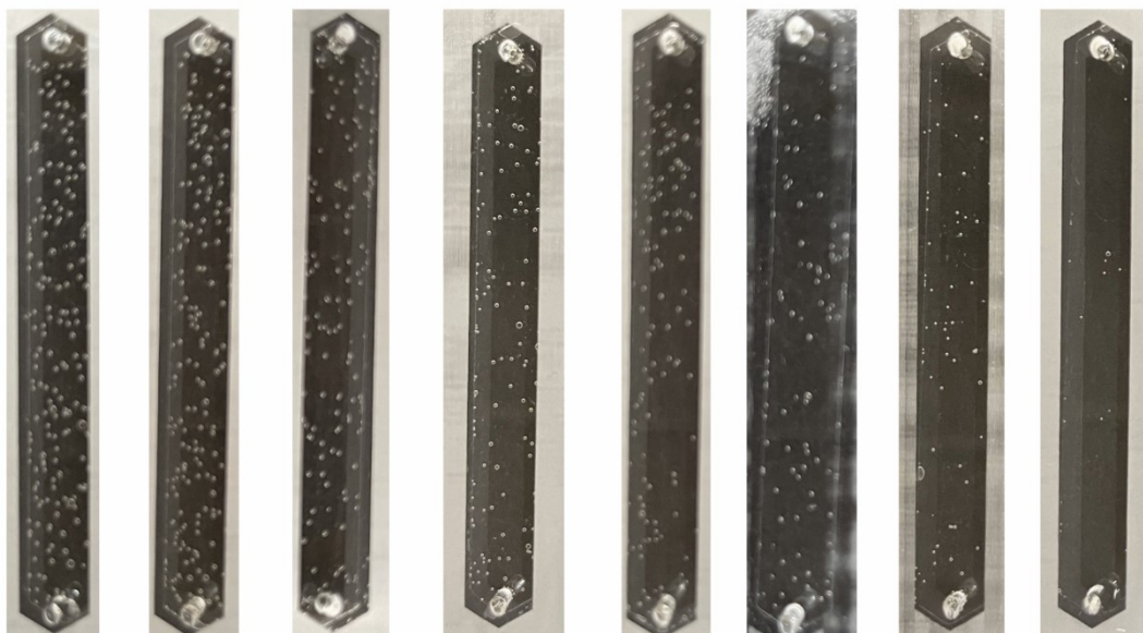
Figure S4. Images of fentanyl bubbling microchips with different concentrations of fentanyl. From left to right: 0, 0.1, 0.5, 1, 2, 5, 10, and 100 ng/mL fentanyl in buffer (PBS, pH 7.4, containing 1% BSA).
