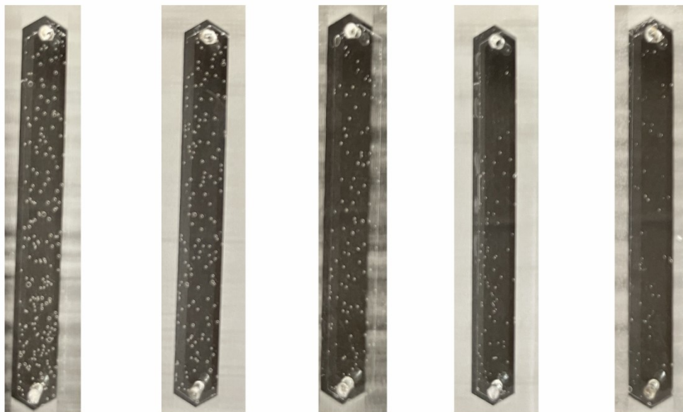
Figure S9. Images of fentanyl bubbling microchips of artificial urine samples with different concentrations of spiked fentanyl. From left to right: artificial urine only, 0.1, 1, 10, and 100 ng/mL spiked fentanyl in artificial urine.
