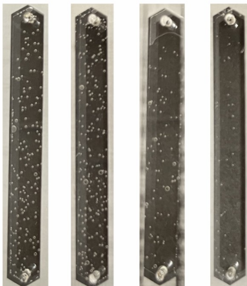
Figure S6. Images of fentanyl bubbling microchips with different concentrations of norfentanyl. From left to right: 0, 10, 100, and 1000 ng/mL norfentanyl in buffer (PBS, pH 7.4, containing 1% BSA).
