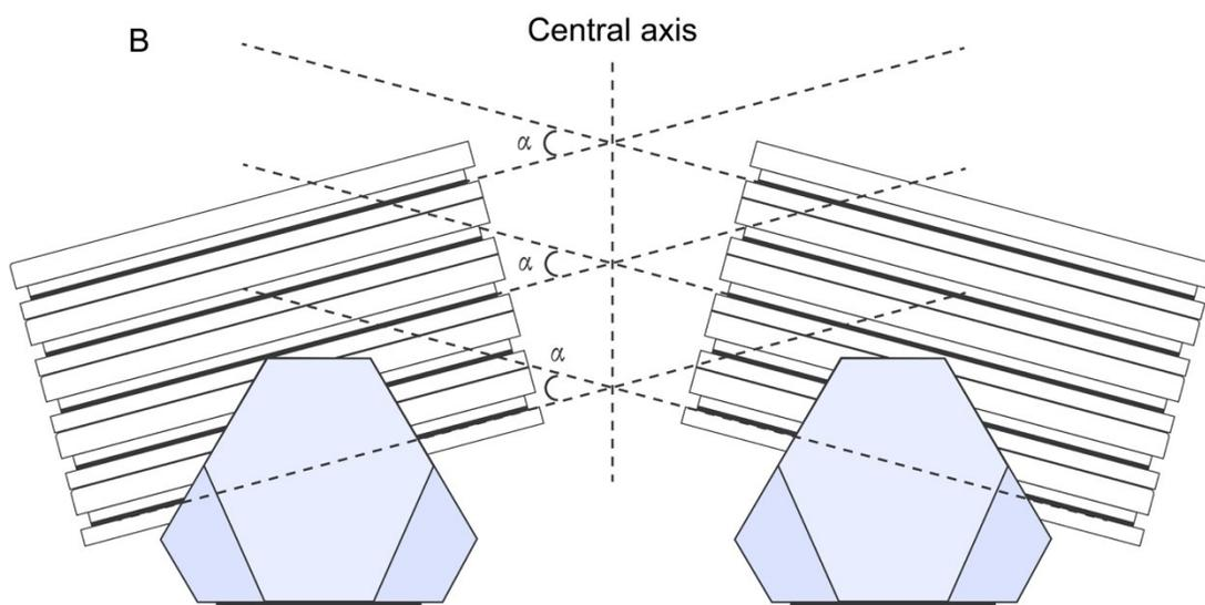
**Fig. S1. Photograph and schematic diagram of the constant-rate flow system with 10 layers of the cPACs stacked onto a rocker.** (A) Photograph of the flow system with 10 layers of the chips. (B) All the chips rotate along the central axis with the same tilting angle ( $\alpha$ ) and frequency.
