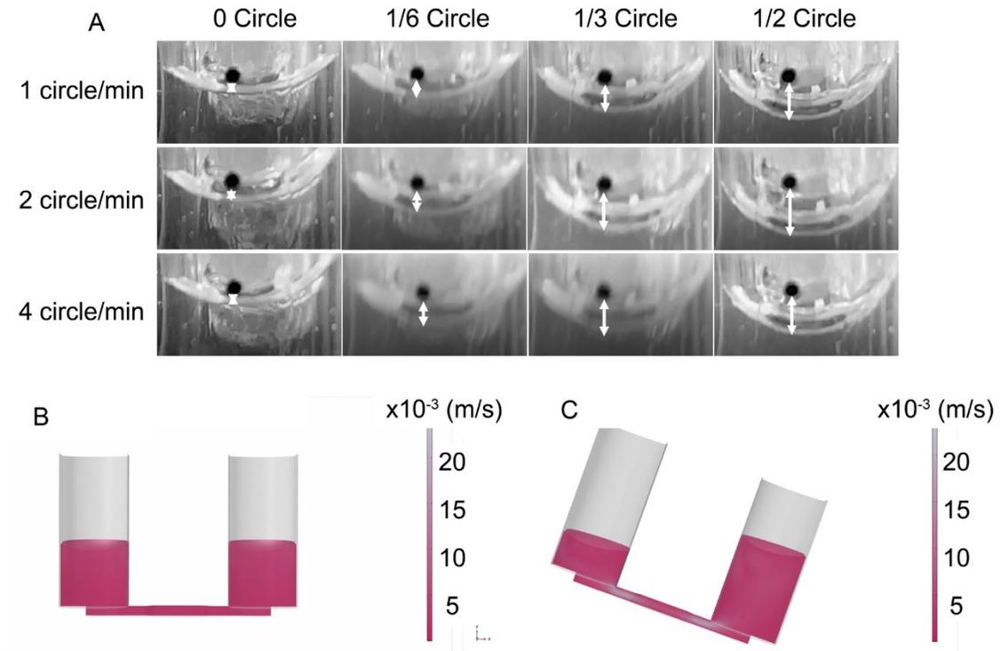
**Fig. S2. The height of the medium in the reservoir changed with the tilting angle. (A)** The photographs showing the height of the medium in the reservoir changed with the tilting angle under different tilting frequencies. (B-C) Simulation of flow rates in the flow channel under the tilting angle of 0 degree (B) and 20 degrees (C), respectively.
