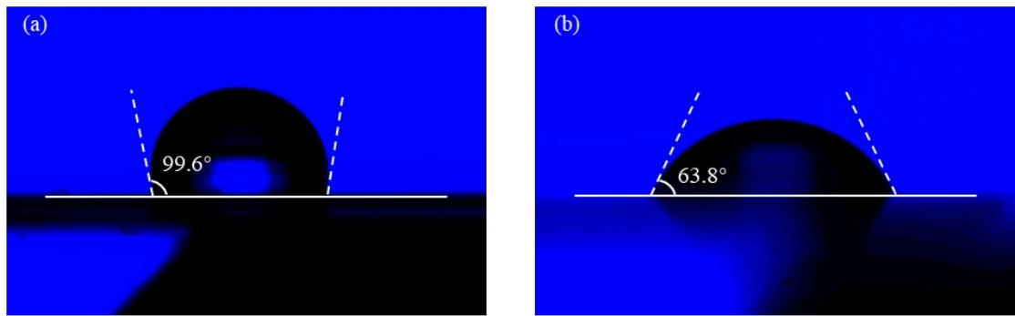
**Figure S2.** Contact angle of water on (a) a SU8 substrate and (b) a silicon substrate.
