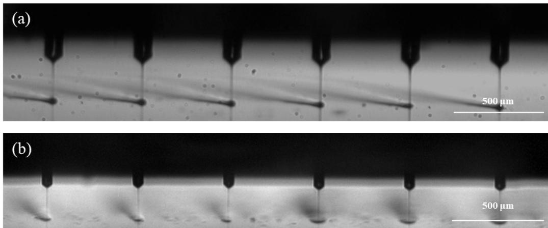
**Figure S10.** The same printhead is capable of printing with different inks. (a) The solution is triethylene glycol; (b) The solution is ethanol.
