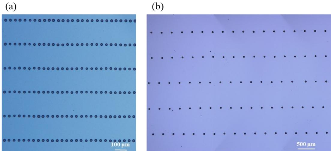
**Figure S12.** (a) Small size droplets ( $< 20$   $\mu\text{m}$ ) printed with triethylene glycol. The printing height is 250  $\mu\text{m}$ , the rectangular pulsed voltage is  $1600 \pm 300$  V, 1000 Hz, 20%; (b) The printed droplets of glycerol. The printing height is 250  $\mu\text{m}$ , the rectangular pulsed voltage is  $1400 \pm 200$  V, 50 Hz, 8%.
