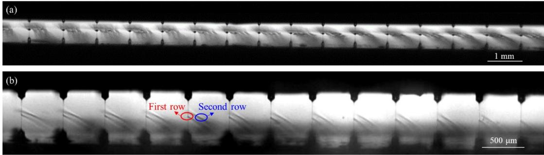
**Figure S8.** (a) The jetting image of an EHD printhead with 24 nozzles, the nozzle spacing is 1mm (limited by the field of vision, only 16 nozzles were photographed). (b) The jetting image of an EHD printhead with a two-row nozzle array, the nozzle spacing is 500  $\mu\text{m}$  (due to the focal length of the camera, only one row of nozzles is photographed. The red and blue ellipses in the figure represent the droplets printed by the first and the second row of nozzles, respectively).
