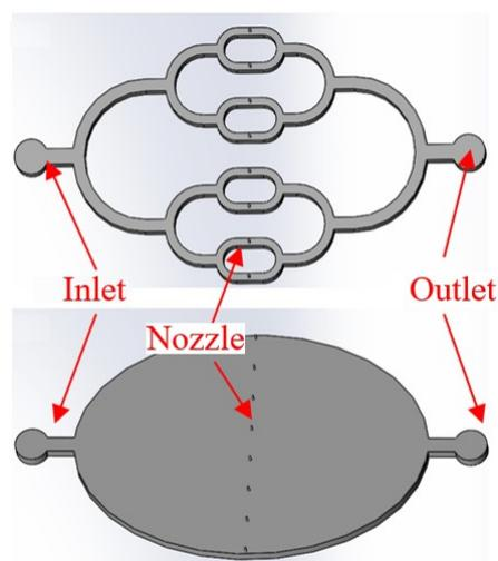
**Figure S4.** The microchannel structure of the printhead chip (back view in Figure 3b in the manuscript).
