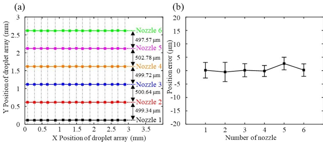
**Figure S9.** (a) Position analysis diagram of droplets in Fig. 4d in the manuscript. (b) Position error analysis of droplet array in Y direction. Take the middle position of nozzles 3 and 4 as the coordinate origin.
