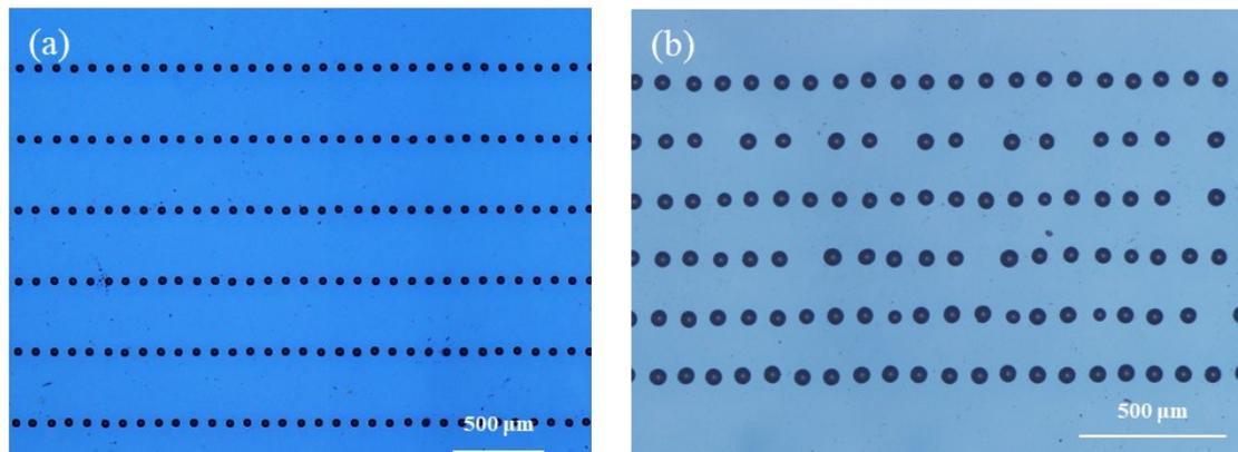
**Figure S7.** (a) The droplets printed by an EHD printhead with  $\Delta x/d_n = 5$  (the nozzle spacing and diameter are 400  $\mu\text{m}$  and 80  $\mu\text{m}$ ) and (b)  $\Delta x/d_n = 2.5$  (the nozzle spacing and diameter are 200  $\mu\text{m}$  and 80  $\mu\text{m}$ ).
