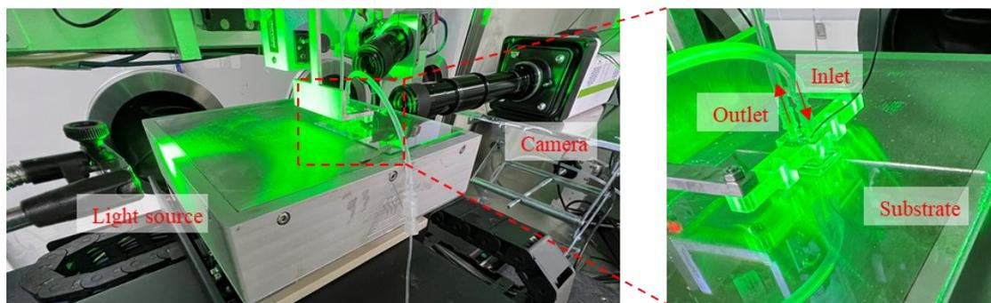
**Figure S6.** The picture of the experimental platform and the printhead.
