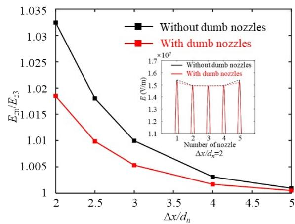
**Figure S3.** The effect of the dumb nozzles on the uniformity of the electric field at the tip of the nozzles.
