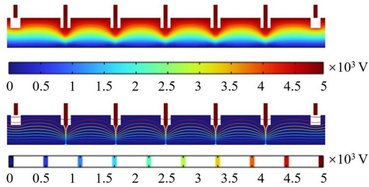
**Figure S5.** The simulation picture of the multi-nozzle EHD printhead with 100  $\mu\text{m}$  nozzle diameter and 500  $\mu\text{m}$  nozzle spacing, which demonstrates that no obvious crosstalk exists.
