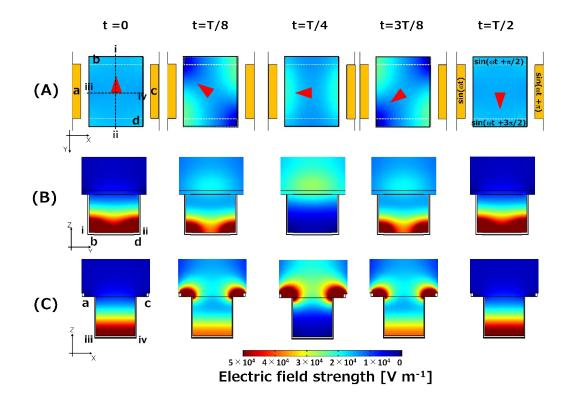
Figure S5. Plot of the electric field strength from the center of the bottom of the microwell to outside of the microwell.
