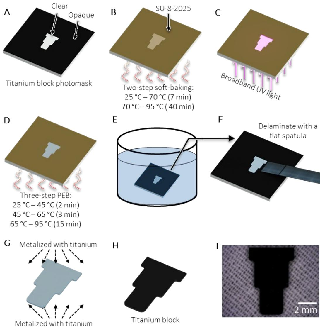
**Figure S3. Schematic diagram for master mold fabrication and the SU-8 master mold used to form titanium blocks.** (A) Chromium-coated photomask. (B) Soft-baking process. (C) Exposure to broadband UV. (D) Post exposure baking process. (E) Immersion into SU-8 developer. (F) Delamination fo SU-8 structure. (G) Metallization of SU-8 structures with titanium. (H) Final titanium block. (I) Picture of fabricate titanium block.
