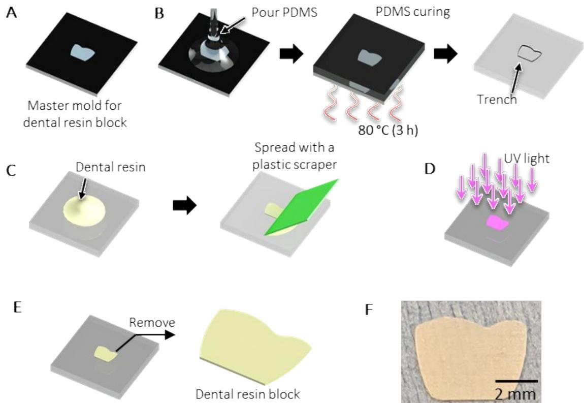
**Figure S1. Schematic for the fabrication of dental resin blocks.** (A) SU-8 master mold for dental resin block. (B) Addition of uncured PDMS to the master mold followed by curing and release of the PDMS layer. (C) Pouring uncured dental resin in the PDMS trench. (D) Curing of dental resin using UV. (E) Removal of dental resin block. (F) Picture of fabricated dental resin block.
