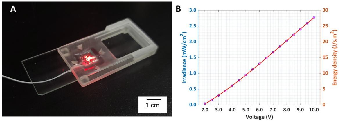
**Figure S4. LED Platform used for PBM therapy.** (A) Glass slide in our custom-chip holder with Red LED. (B) Irradiance profile of platform.
