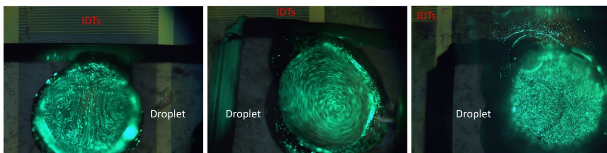
Figure S12. Acoustic streaming in the droplet (a) entirely present on SAW propagation path, (b) partially present on SAW propagation path, and (c) absent on SAW propagation path.
