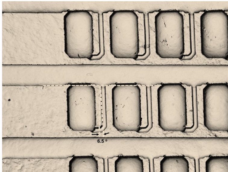
Figure S5. Image of a COP sheet following hot embossing with a PDMS-investment powder mold without an aluminum frame, showing distortion of fine features: drainage channels are at a 6.5^\circ angle from perpendicular to the main channel.
