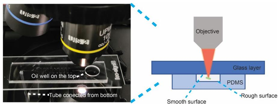
**Fig. S1** The setup of the OPSI Chip on the EasySort stage. The laser would penetrate the upper glass layer and reach the cell in the channel on the PDMS layer. As the glass layer features a smoother surface than PDMS channel wall, the bottom set PDMS design can achieve a stronger optical tweezers force.
