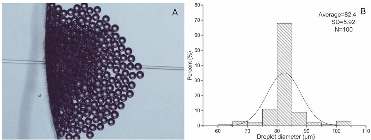
**Fig. S3 Continuous droplet generation for the verification of size uniformity. (A) Droplets generated in the oil well. (B) Distribution of diameters of the 100 droplets generated.**
