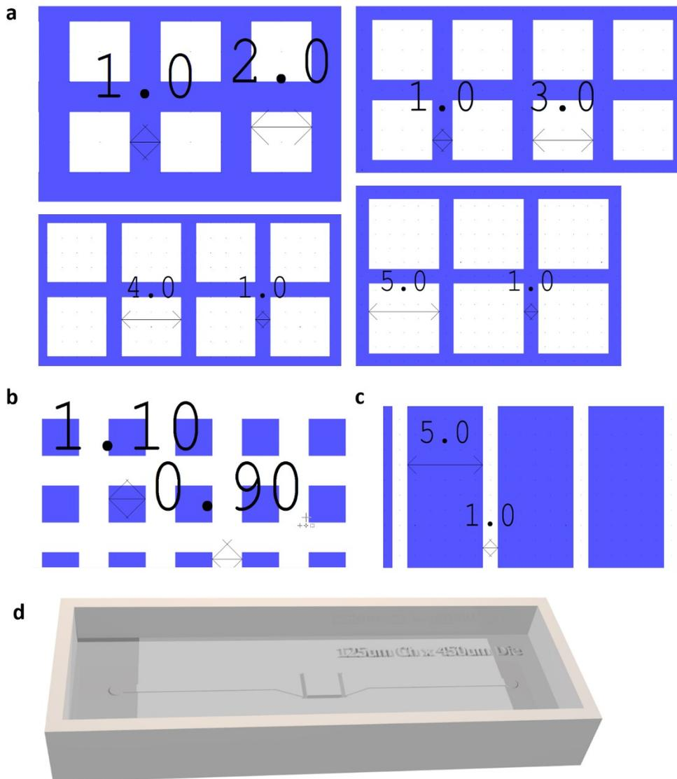
Supplementary FIG. S1. Summary of designs used for fabrication. (a) Four different layouts of KOH pyramids; (b) Pillars and Cryo pyramids; (c) Ridges; and (d) 3D printed mold to cast soft microfluidic device.
