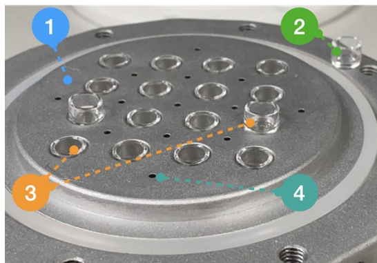
Fig. S2. Graph of the multi-sample holding module. (1) sample-holding array sheet, which also worked as the GE. (2) The glass receptacles. (3) Glass receptacles in the holding wells. (4) Exhaust vents (The surplus gases flow out of the device through those vents).
