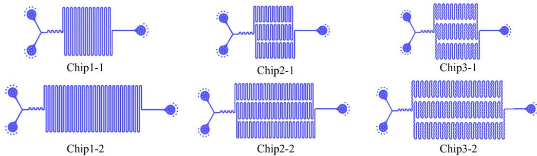
**Fig. S3** The schematic diagram of the six types of chips. Each chip contains two inlets and one outlet. The microchannel length of Chip 1-1, Chip 2-1 and Chip 3-1 was about 25 cm. The microchannel length of Chip 1-2, Chip 2-2 and Chip 3-2 was nearly 50 cm.
