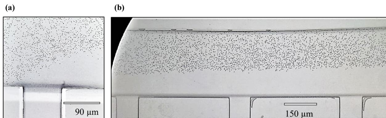
Fig. S1 Experimental observation of the exclusion zone formation in dead-end channel for pore width = 100  $\mu\text{m}$ . (a) For 1  $\mu\text{m}$  silica particles at  $t=3\text{min}$  over the first pore. (b) For 2  $\mu\text{m}$  silica particles at  $t=3\text{min}$  over pores 4 to 6.
