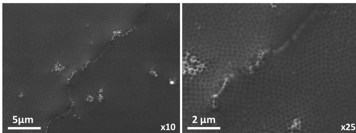
**Figure S6.** SEM images after the infiltration of the PS-NS template and conversion of the metal xanthates to  $\text{CuInS}_2$  at  $195\text{ }^\circ\text{C}$ .
