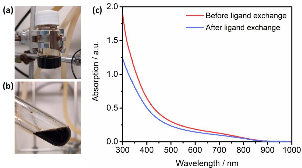
**Figure S12.** Digital photos of the (a) dioleamide-capped CuInS<sub>2</sub> nanocrystals dispersed in toluene and (b) thioglycerol-capped CuInS<sub>2</sub> nanocrystals dispersed in DMSO. (c) UV-Vis spectra of the CuInS<sub>2</sub> nanocrystals before and after ligand exchange.
