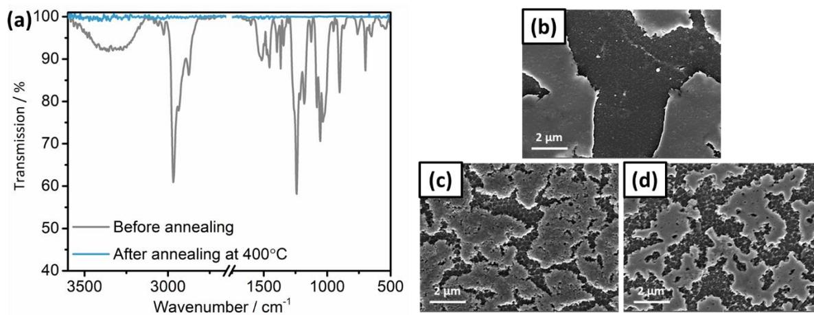
**Figure S7.** (a) FT-IR spectra after infiltration of the PS-NS template with the precursor solution (grey) and after annealing at  $400\text{ }^\circ\text{C}$  (blue) of initial attempts using a too high precursor concentration. SEM images of (b) CIS-P0, (c) CIS-P300 and (d) CIS-P600 after annealing at  $400\text{ }^\circ\text{C}$ .
