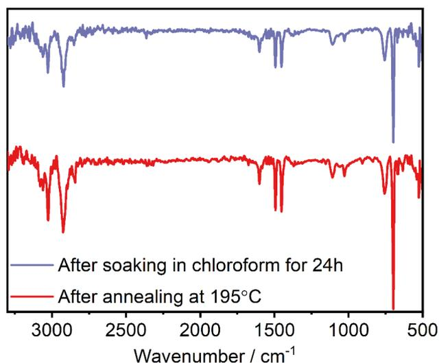
**Figure S10.** FT-IR spectra of films after annealing at 195 °C (lower spectrum) and after soaking of the sample in chloroform for 24 h, for PS-MS template dissolution (upper spectrum). The spectra are shifted vertically for better visibility.
