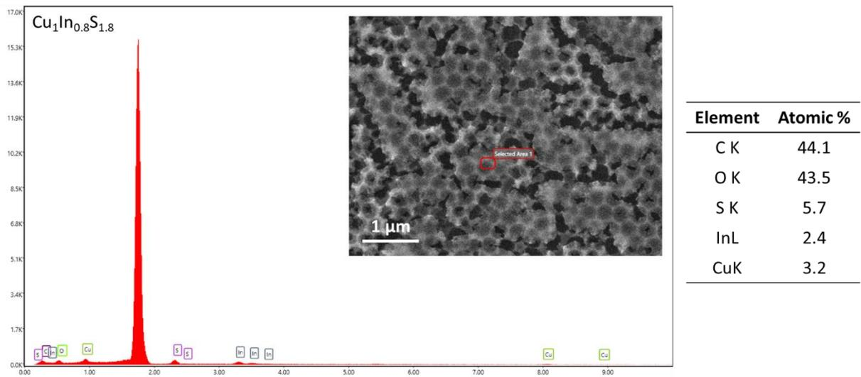
**Figure S2.** EDX spectrum obtained from the CIS-P600 sample after annealing at 400 °C. The measurement was performed directly on the film.
