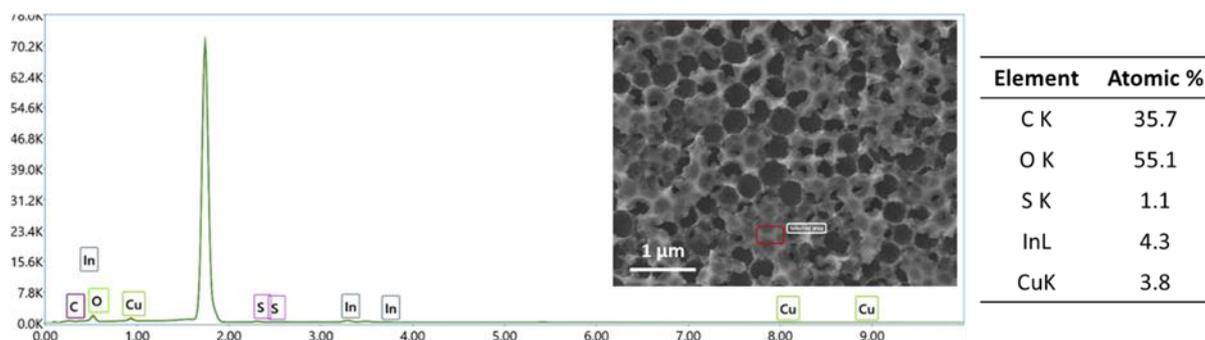
**Figure S9.** EDX spectrum obtained from the CIS-P600 sample after thermal oxidation at 280 °C. The measurement was performed directly on the film.
