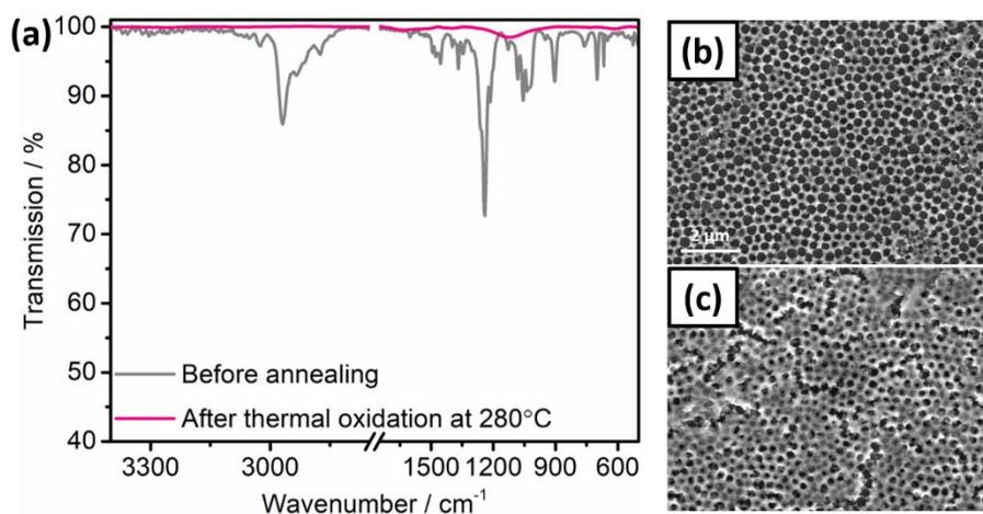
**Figure S8.** (a) FT-IR spectra after infiltration of the PS-NS template with the precursor solution (grey) and after the thermal oxidation process at 280 °C (pink). SEM images of (b) CIS-P300 and (c) CIS-P600 after thermal oxidation at 280 °C.
