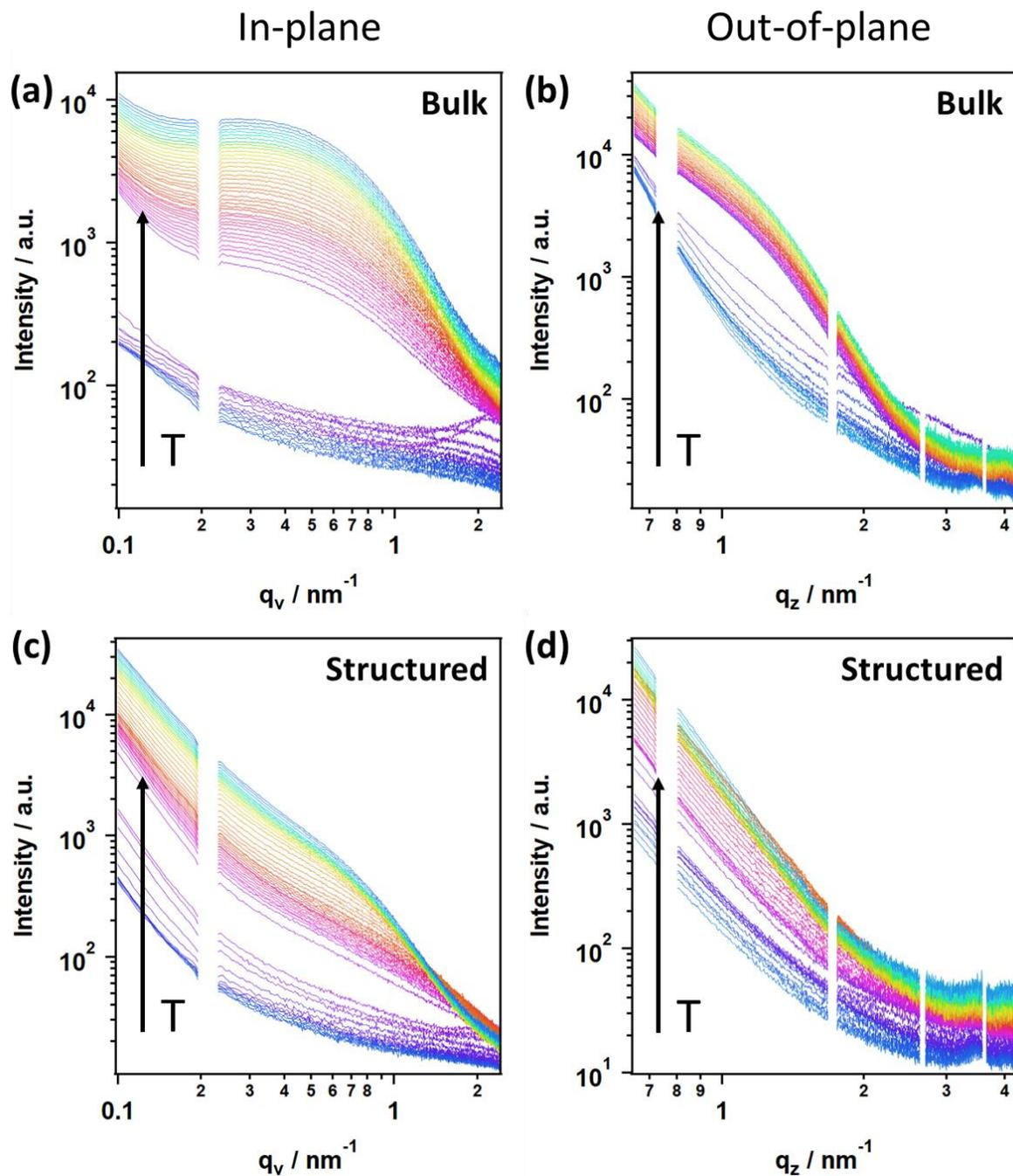
**Figure S4.** Temperature-dependent development of the (a) in-plane and (b) out-of-plane GISAXS patterns of the bulk film (non-structured) and temperature-dependent development of the (c) in-plane and (d) out-of-plane GISAXS patterns of the structured film. The increasing temperature (T) is indicated with a black arrow in the graphs. The data are shifted vertically for better visibility.
