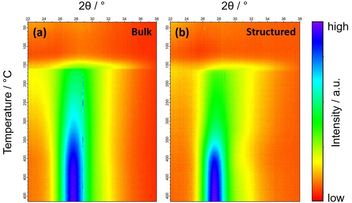
**Figure S5.** GIWAXS surface plots of (a) a bulk and (b) a structured film measured between 22 and 38° 2θ during heating runs from 35 up to 400 °C with a heating rate of 10 °C/min and a subsequent annealing time of 15 min at 400 °C.
