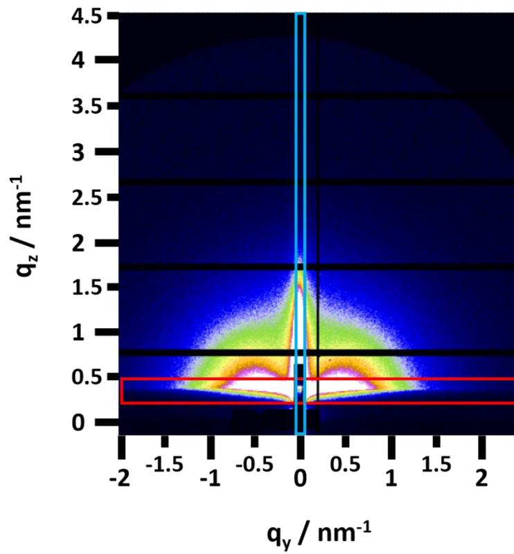
**Figure S3.** Analysis of the GISAXS data; the blue and red boxes enclose the out-of-plane and in-plane integration areas, respectively.
