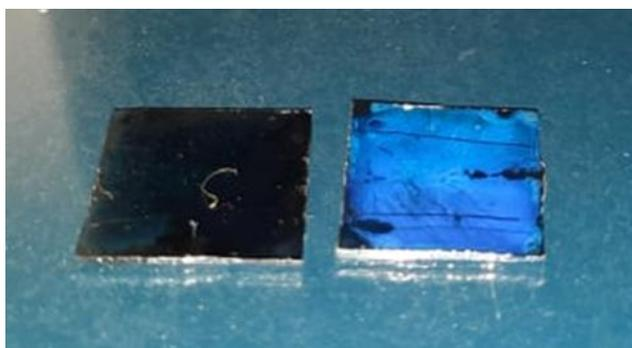
**Figure S13.** Digital photo of the films before (left) and after (right) template removal (nanocrystal ink route).
