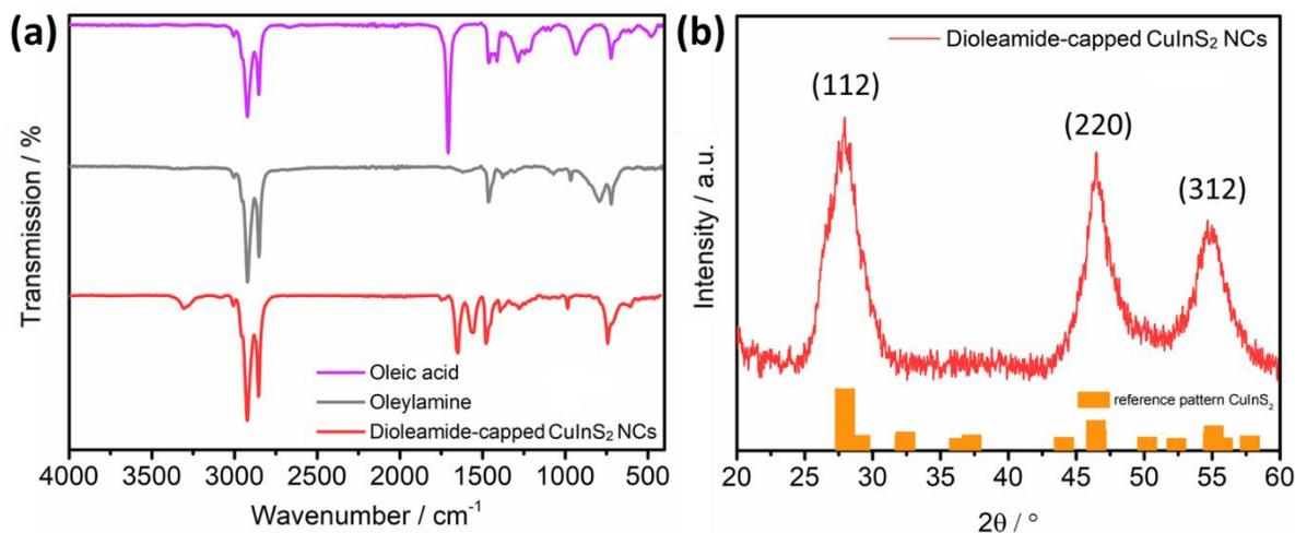
**Figure S11.** (a) FT-IR spectra of dioleamide-capped  $\text{CuInS}_2$  NCs (red spectrum), free oleylamine (grey spectrum) and free oleic acid (purple spectrum). The spectra are shifted vertically for better visibility. (b) X-ray diffraction pattern of  $\text{CuInS}_2$  before ligand exchange, with a reference pattern for chalcopyrite  $\text{CuInS}_2$  (ICSD-42127).
