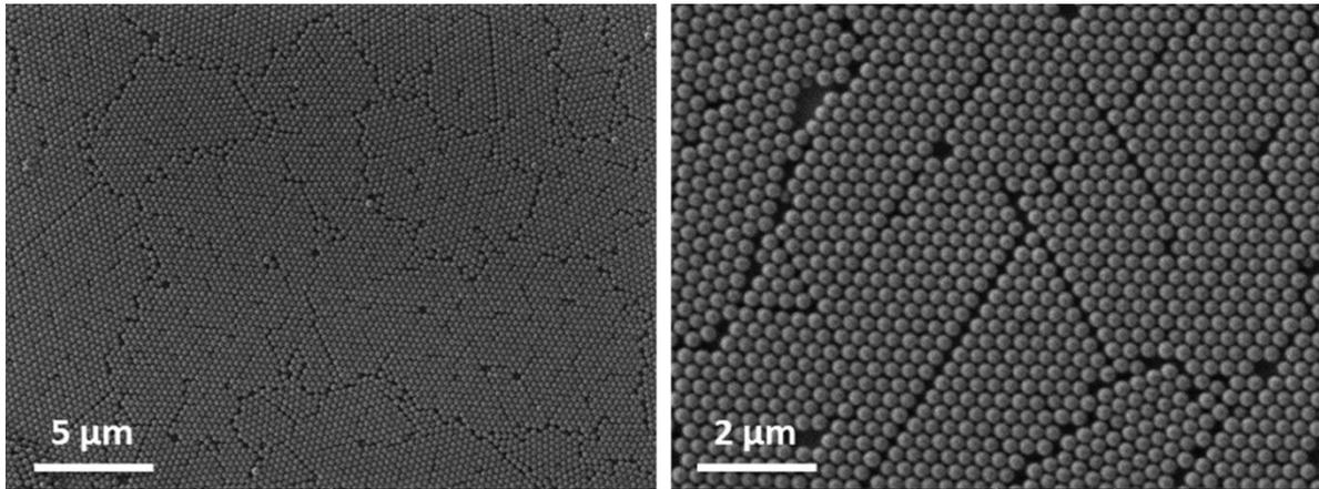
**Figure S1.** SEM images of the PS-MS templates prepared with an air/liquid interface method in two different magnifications.
