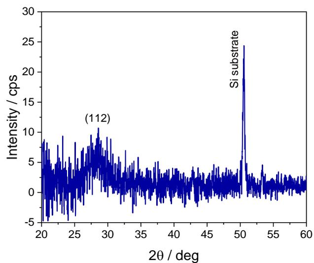
**Figure S14.** GIXRD pattern of a 75 nm thick honeycomb structured CuInS<sub>2</sub> film on a silicon substrate prepared via the nanocrystal ink route.
