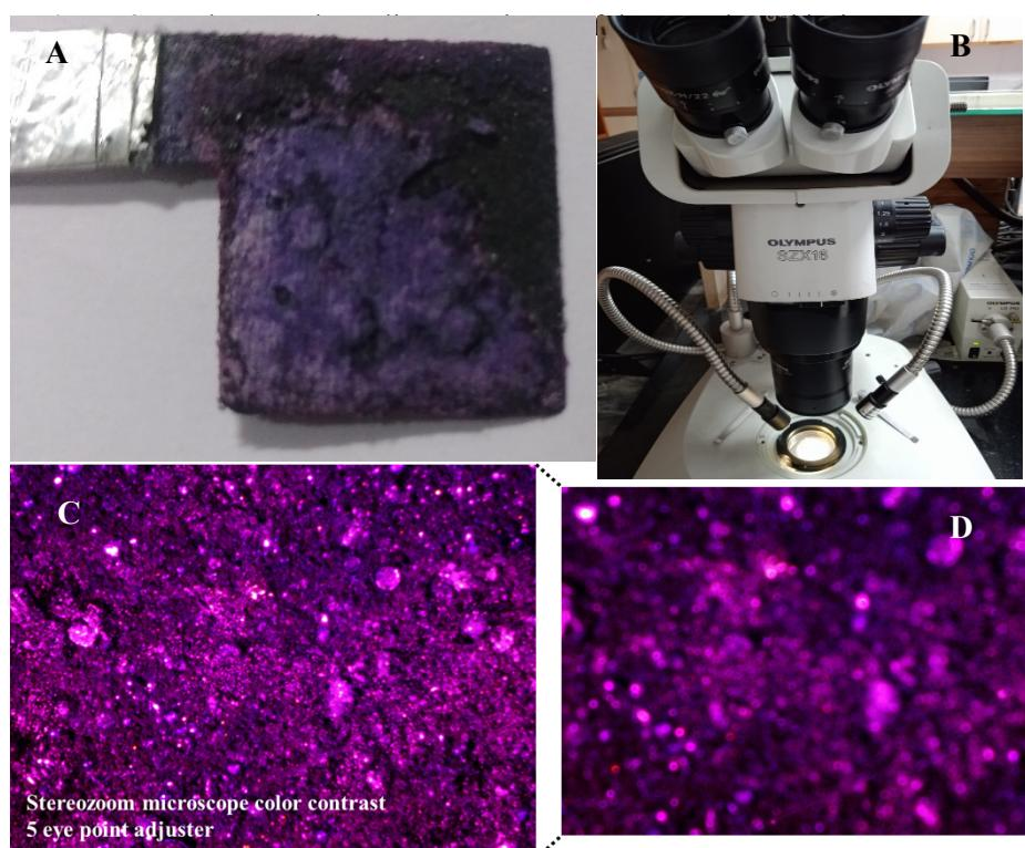
**Figure S8.** A) shows the surface genuine color of the electrode after cycling experiment, fully charged. B) shows the visual image of the optical microscope with magnifying lenses, illuminators, stereo zoom adjuster and camera. C&D) The electrode surface under stereozoom optical microscope. maximized color contrast image where the coral like structures were visible.
