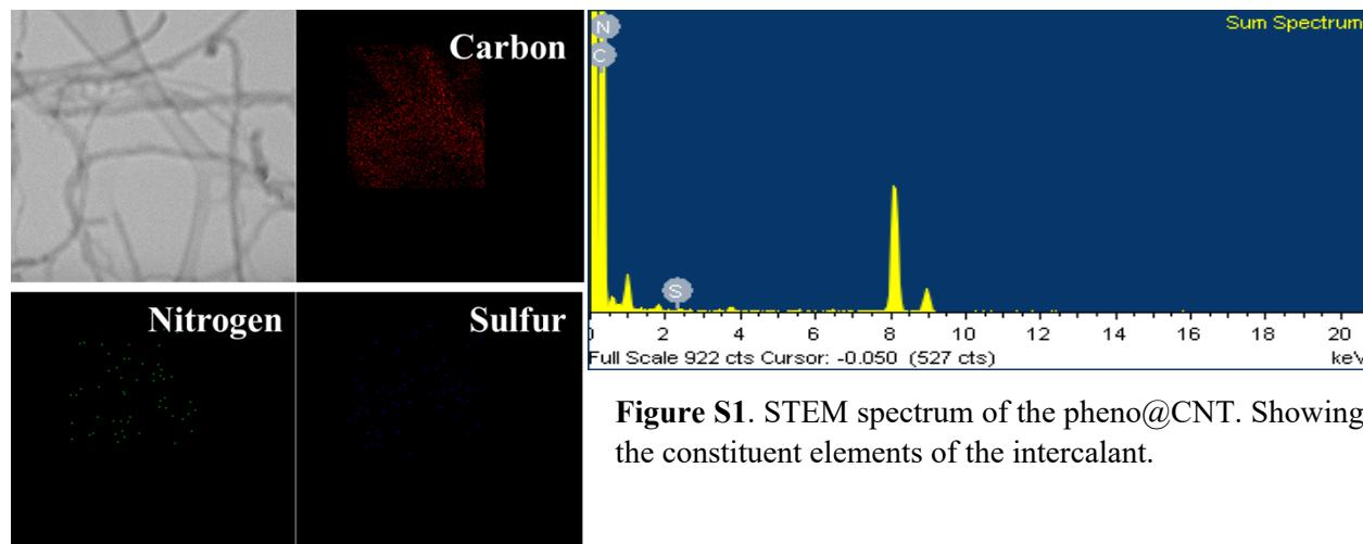
**Figure S1.** STEM spectrum of the pheno@CNT. Showing the constituent elements of the intercalant.
