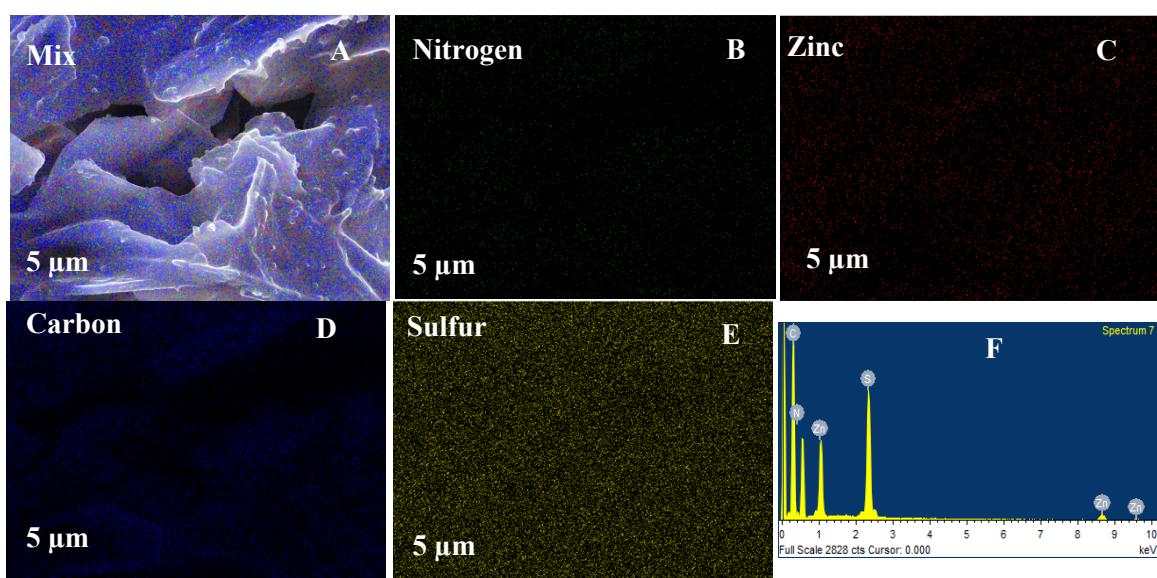
**Figure S10.** Shows the EDX elemental mapping of the cathode with neat phenothiazine. A) Mix, B) Nitrogen, C) Zinc, D) Carbon, E) Sulfur, F) EDX elemental mapping spectrum of the cathode.
