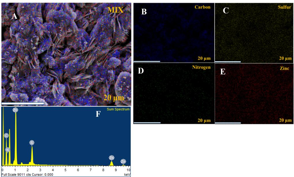
**Figure S11.** Shows the EDX elemental mapping of the cathode with pheno@CNT after cycling experiment. A) Mix, B) Carbon, C) Sulfur, D) Nitrogen, E) Zinc F) EDX spectrum. (The high amount of sulphur indicated the sulphate anion intercalation into the cathode).
