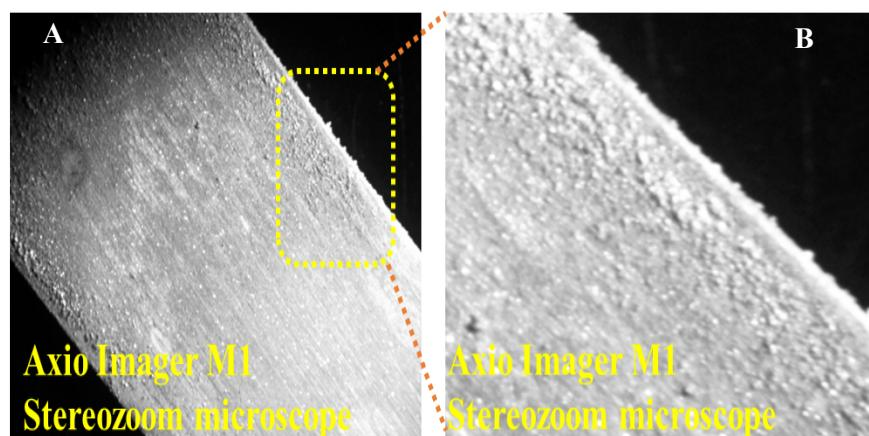
**Figure S12.** Stereozoom optical microscopic images of anode at zoom range A) 7x and B) 11x.
