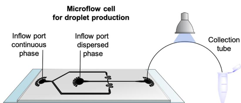
**Figure SI-2.** Scheme of the experimental setup for PAG microgel fabrication. AutoCAD sketch of a microflow cell for droplet generation connected via tubing to an Eppendorf collection vial, in which the formed emulsion is collected. The emulsion is irradiated in the outflow tubing with UV light directly from the light guide of a UV source. Details regarding the UV source can be found in the Materials and methods section.
