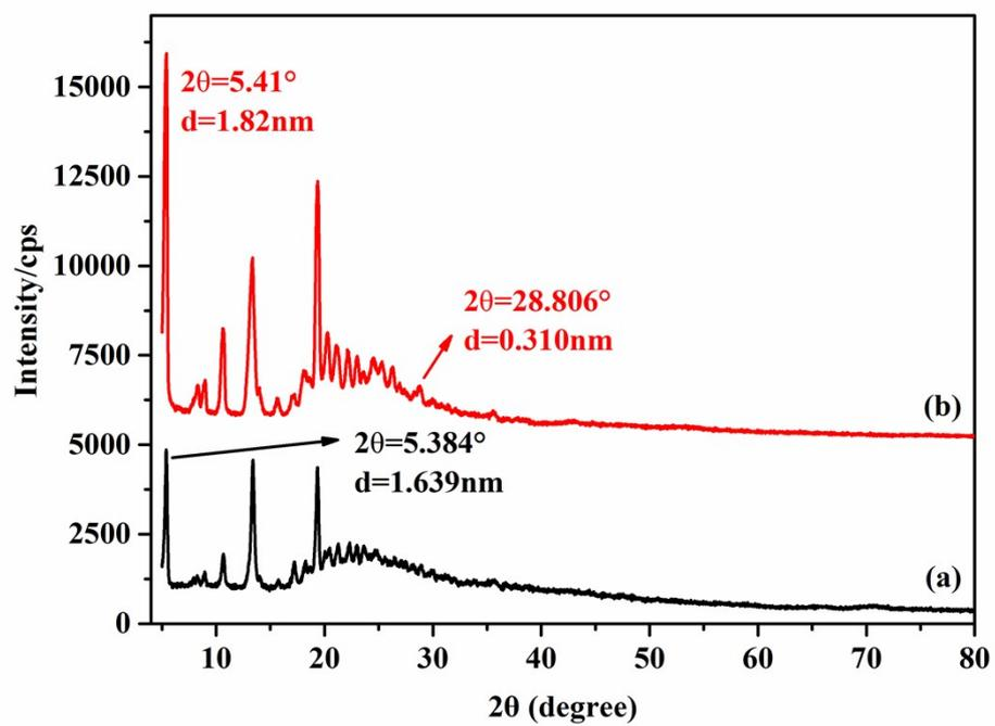
**Fig. S6** XRD of the gelator G3 (a) and G3-Mg<sup>2+</sup> complex (b)
