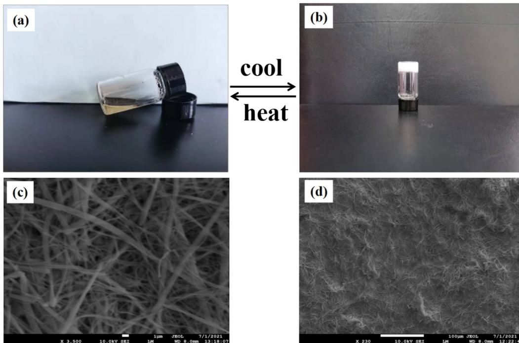
**Fig. S13.** a,b) the reversible gel-sol transformation of the G3-gel by temperature;
