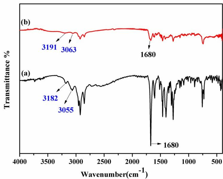
**Fig. S4** FT-IR spectra of the gelator G3 (a) and G3-Mg<sup>2+</sup> complex (b)
