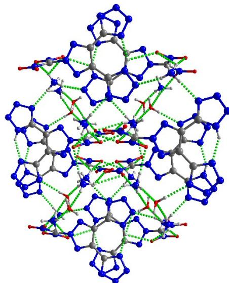
**Figure S4.** Crystal packing of **5a·H<sub>2</sub>O** view c axis
