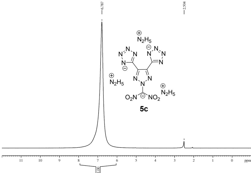
**Figure S22.**  $^1\text{H}$  NMR-Compound **5c**
