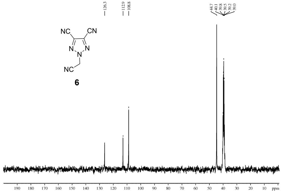
**Figure S25.**  $^{13}\text{C}$  NMR-Compound **6**
