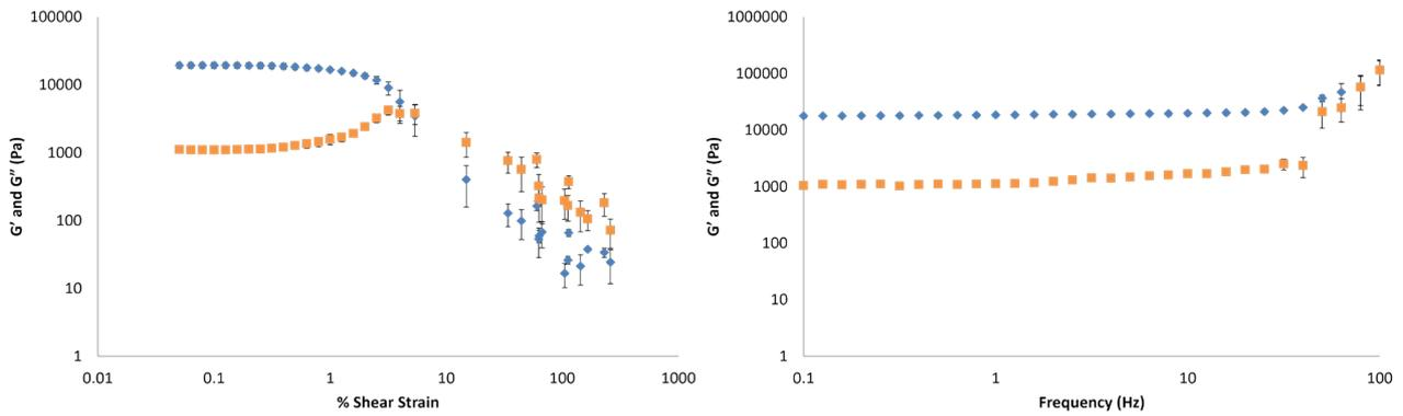
Figure S35. Elastic ( $G'$ , blue circles) and viscous ( $G''$ , red circles) moduli of DBS-CONHNH<sub>2</sub>/gellan gum hydrogel (0.3% wt/vol DBS-CONHNH<sub>2</sub> and 0.5% wt/vol gellan gum) prepared with 0.15% wt/vol CaCO<sub>3</sub> and 1.0% wt/vol GdL with increasing shear strain (left) and frequency (right).
