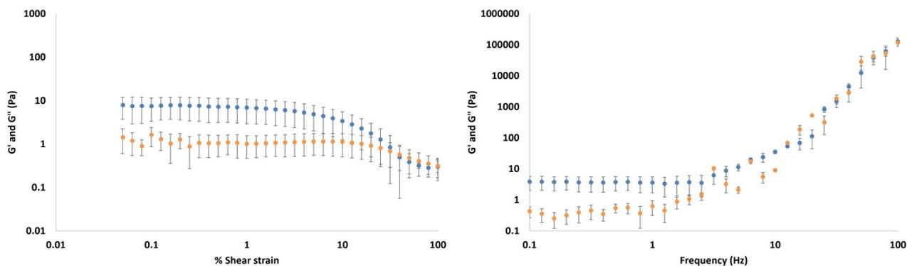
Figure S51. Elastic ( $G'$ , blue circles) and viscous ( $G''$ , red circles) moduli of DBS-CONH<sub>2</sub> hydrogel (0.4% wt/vol - loaded with 1 mL AgNO<sub>3</sub> 10 mM) with increasing shear strain (left) and frequency (right).
