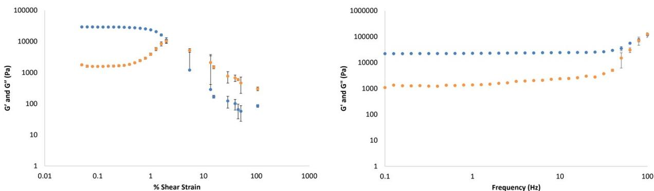
Figure S16. Elastic ( $G'$ , blue circles) and viscous ( $G''$ , orange circles) moduli of DBS-CONH<sub>2</sub>/gellan gum multicomponent hydrogel (0.3% wt/vol DBS-CONH<sub>2</sub> and 0.5% wt/vol gellan gum) with increasing shear strain (left) and frequency (right).
