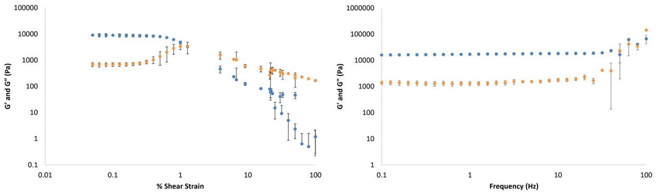
Figure S13. Elastic ( $G'$ , blue circles) and viscous ( $G''$ , orange circles) moduli of gellan gum hydrogel (1.3% wt/vol) with increasing shear strain (left) and frequency (right).
