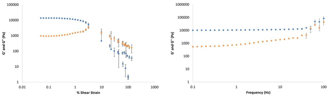
Figure S15. Elastic ( $G'$ , blue circles) and viscous ( $G''$ , orange circles) moduli of DBS-CONH<sub>2</sub>/gellan gum multicomponent hydrogel (0.3% wt/vol of both gelators) with increasing shear strain (left) and frequency (right).
