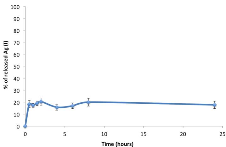
Figure S47. Release over time of Ag(I) ions from DBS-CONHNH<sub>2</sub>/gellan gum hybrid gel beads loaded with Ag NPs.
