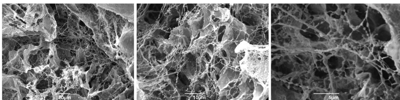
Figure S44. SEM images of photoactivated DBS-CONH<sub>2</sub>NH<sub>2</sub>/gellan gum prepared using CaCO<sub>3</sub> as a cross-linker and DPIN as a pH activator. Scale bars (from left to right): 10 μm (left and centre) and 5 μm (right).
