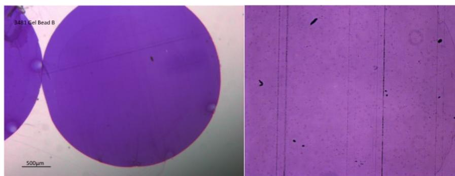
Figure S23. Optical microscopy image of DBS-CONH<sub>2</sub>/gellan gum gel bead embedded in resin and stained with toluidine blue.
