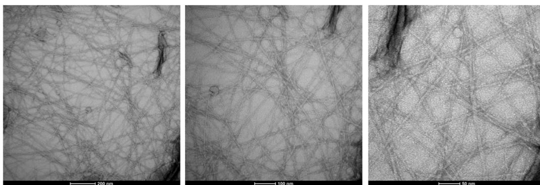
Figure S41. TEM image of photoactivated gellan gum gel prepared using  $\text{CaCO}_3$  as a cross-linker and DPIN as a pH activator. Scale bars (from left to right): 200 nm, 100 nm and 50 nm.
