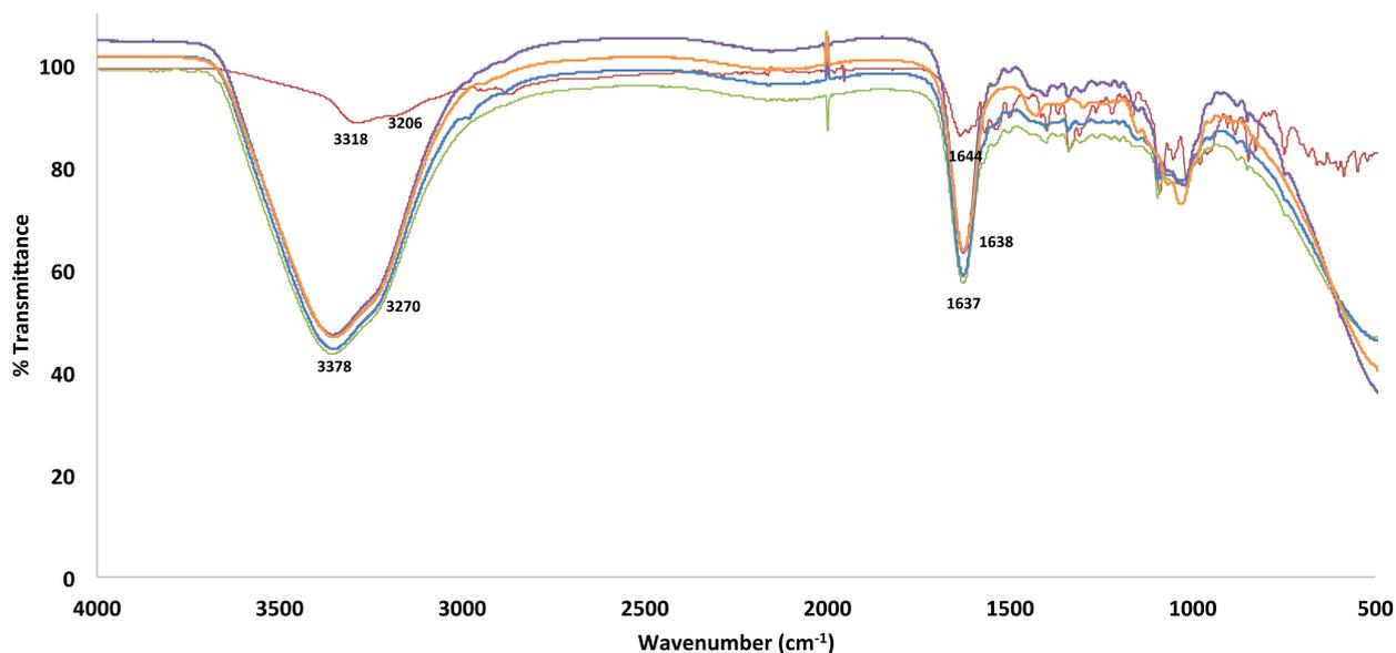
Figure S3. IR spectra of xerogels obtained from DBS-CONH $_2$  gel (0.4% wt/vol, red line), gellan gum gel (1.3% wt/vol, orange line) and DBS-CONH $_2$ /gellan gum two-component gel cross-linked with CaCl $_2$ , containing 0.3% wt/vol of DBS-CONH $_2$  and 0.3% wt/vol gellan gum (green line), 0.5% wt/vol gellan gum (blue line) and 1.0% wt/vol gellan gum (purple line).
