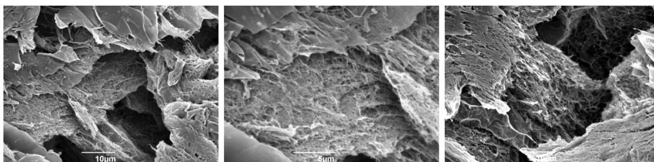
Figure S43. SEM images of photoactivated gellan gum prepared using CaCO<sub>3</sub> as a cross-linker and DPIN as a pH activator. Scale bars (from left to right): 10, 5 and 1 μm.
