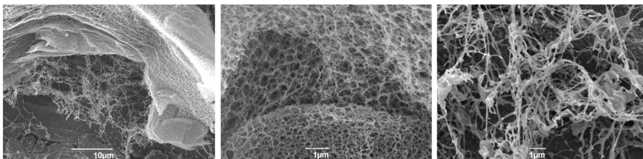
Figure S29. SEM images of gellan gum gel prepared using CaCO<sub>3</sub> as a cross-linker and GdL as a pH activator. Scale bars: 10 μm (left) and 1 μm (centre and right).
