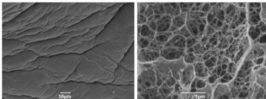
Figure S7. SEM images of DBS-CONH<sub>2</sub>/gellan gum gel bead cross-section (cross-linked with CaCl<sub>2</sub>). Scale bars: 10 (left) and 1 μm (right).
