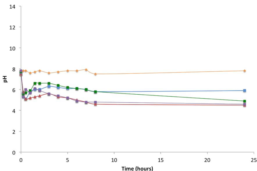
Figure S18. pH changes over time during the formation of the DBS-CONH<sub>2</sub> gel (0.3% wt/vol, orange line) and DBS-CONH<sub>2</sub>/gellan gum hybrid gels (CaCO<sub>3</sub> - 0.15% wt/vol and GdL - 0.8% wt/vol) containing: 0.3% wt/vol of DBS-CONH<sub>2</sub> and 0.1% wt/vol gellan gum (blue line), 0.3% wt/vol gellan gum (red line), 0.5% wt/vol gellan gum (green line) or 1.0% wt/vol gellan gum (purple line).
