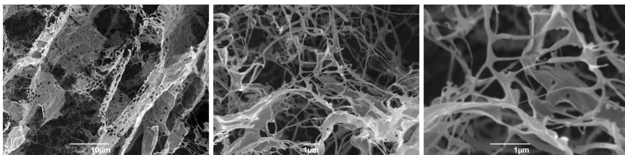
Figure S27. SEM images of DBS-CONHNH<sub>2</sub>/gellan gum gel bead cross-section (prepared using CaCO<sub>3</sub> as a cross-linker and GdL as a pH activator). Scale bars (from left to right): 10 (left) and 1 μm (centre and right).
