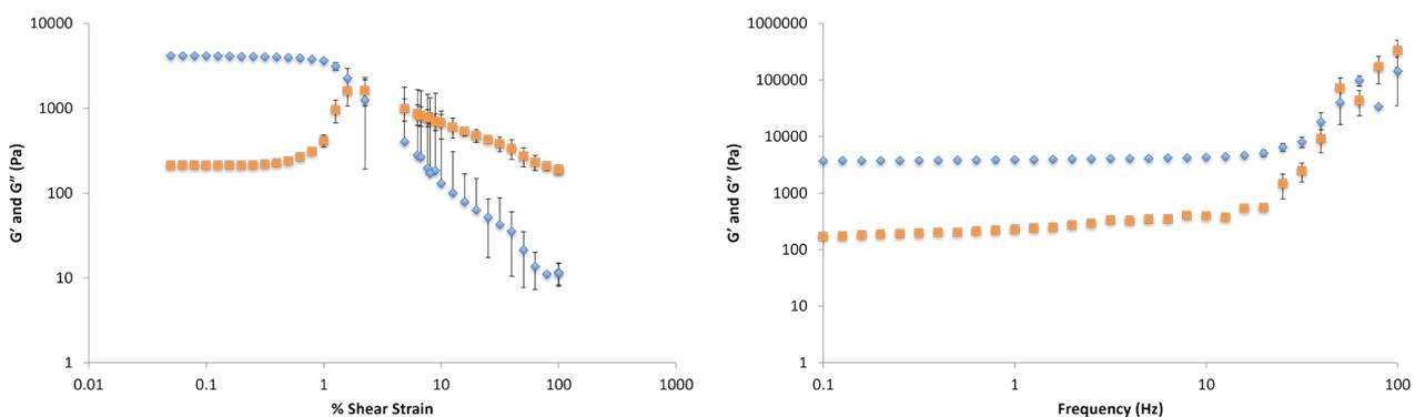
Figure S55. Elastic ( $G'$ , blue circles) and viscous ( $G''$ , red circles) moduli of gellan gum hydrogel (0.6% wt/vol– loaded with 1 mL AgNO<sub>3</sub> 10 mM) with increasing shear strain (left) and frequency (right).
