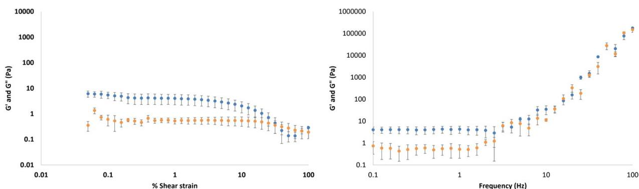
Figure S52. Elastic ( $G'$ , blue circles) and viscous ( $G''$ , red circles) moduli of DBS-CONH<sub>2</sub> hydrogel (0.4% wt/vol - loaded with 3 mL AgNO<sub>3</sub> 10 mM) with increasing shear strain (left) and frequency (right).
