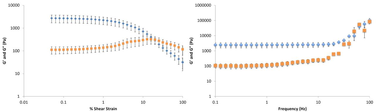
Figure S33. Elastic ( $G'$ , blue circles) and viscous ( $G''$ , red circles) moduli of DBS-CONH<sub>2</sub>/gellan gum hydrogel (0.3% wt/vol DBS-CONH<sub>2</sub> and 0.1% wt/vol gellan gum) prepared with 0.15% wt/vol  $\text{CaCO}_3$  and 1.0% wt/vol GdL with increasing shear strain (left) and frequency (right).
