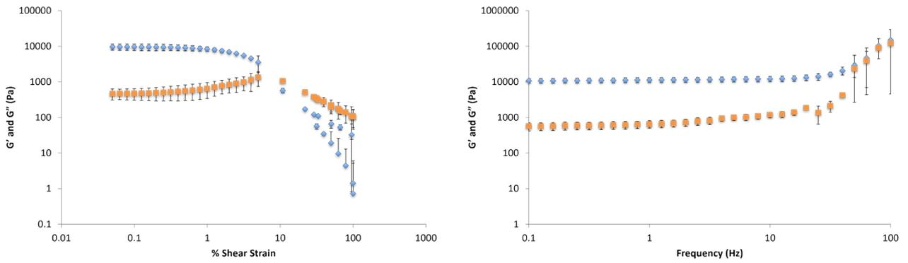
Figure S53. Elastic ( $G'$ , blue circles) and viscous ( $G''$ , red circles) moduli of DBS-CONH<sub>2</sub>/gellan gum hydrogel (0.3% wt/vol DBS-CONH<sub>2</sub> and 0.3% wt/vol gellan gum – loaded with 1 mL AgNO<sub>3</sub> 10 mM) with increasing shear strain (left) and frequency (right).
