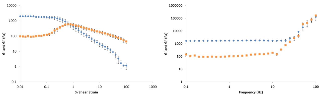
Figure S30. Elastic ( $G'$ , blue circles) and viscous ( $G''$ , red circles) moduli of gellan gum hydrogel (0.4% wt/vol) prepared with 0.15% wt/vol CaCO<sub>3</sub> and 0.8% wt/vol GdL with increasing shear strain (left) and frequency (right).
