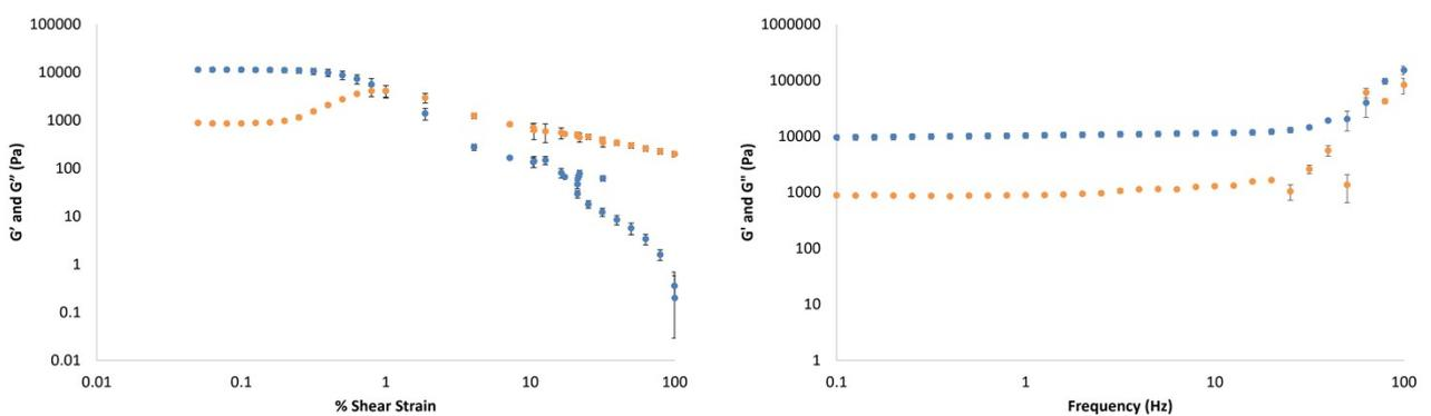
Figure S12. Elastic ( $G'$ , blue circles) and viscous ( $G''$ , orange circles) moduli of gellan gum hydrogel (0.8% wt/vol) with increasing shear strain (left) and frequency (right).
