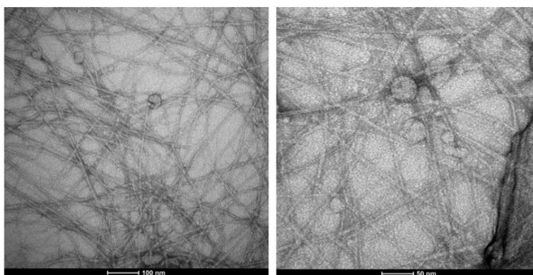
Figure S25. TEM images of gellan gum gel prepared using CaCO<sub>3</sub> as a cross-linker and GdL as a pH activator. Scale bars from left to right: 100 and 50 nm.
