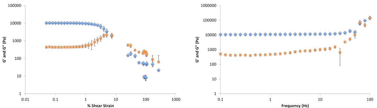
Figure S34. Elastic ( $G'$ , blue circles) and viscous ( $G''$ , red circles) moduli of DBS-CONH<sub>2</sub>/gellan gum hydrogel (0.3% wt/vol DBS-CONH<sub>2</sub> and 0.3% wt/vol gellan gum) prepared with 0.15% wt/vol  $\text{CaCO}_3$  and 1.0% wt/vol GdL with increasing shear strain (left) and frequency (right).
