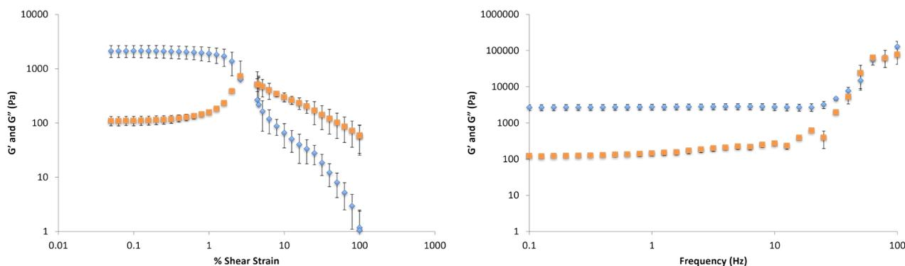
Figure S56. Elastic ( $G'$ , blue circles) and viscous ( $G''$ , red circles) moduli of gellan gum hydrogel (0.6% wt/vol– loaded with 3 mL  $\text{AgNO}_3$  10 mM) with increasing shear strain (left) and frequency (right).
