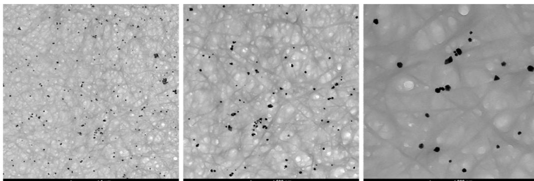
Figure S48. TEM images of DBS-CONH<sub>2</sub> gel incorporating AgNPs. Scale bars (from left to right): 1 μm, 500 nm and 200 nm.
