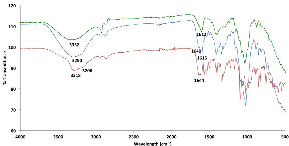
Figure S22. IR spectra of xerogels obtained from DBS-CONH<sub>2</sub> gel (0.4% wt/vol, red line), gellan gum gel (0.8% wt/vol, green line) and DBS-CONH<sub>2</sub>/gellan gum gel containing 0.3% wt/vol of DBS-CONH<sub>2</sub> and 0.5% wt/vol gellan gum (green line).
