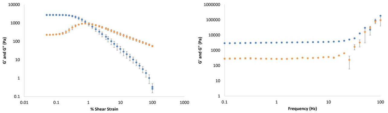
Figure S10. Elastic ( $G'$ , blue circles) and viscous ( $G''$ , orange circles) moduli of gellan gum hydrogel (0.4% wt/vol) with increasing shear strain (left) and frequency (right).
