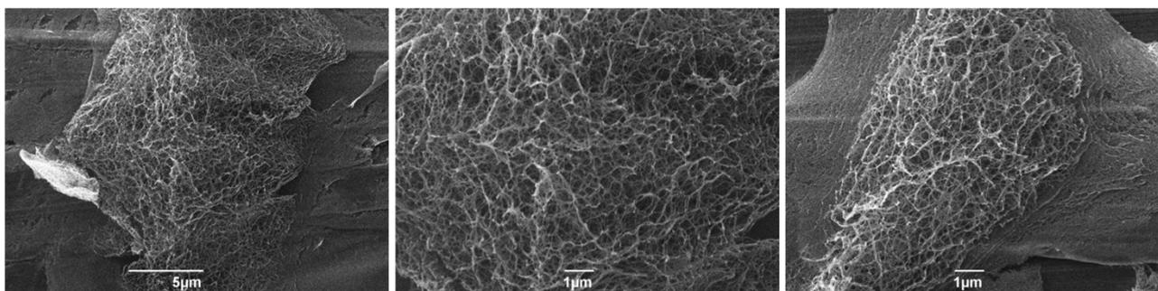
Figure S8. SEM images of gellan gum gel cross-linked with CaCl<sub>2</sub>. Scale bars (from left to right): 5 (left) and 1 μm (centre and right).
