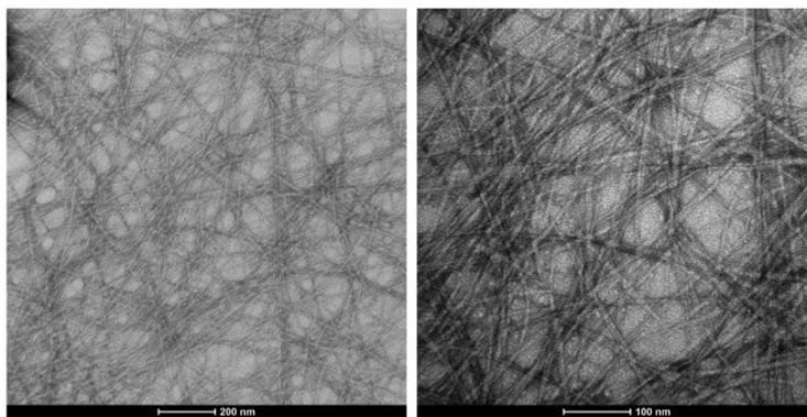
Figure S24. TEM images of DBS-CONHNH<sub>2</sub>/gellan gum hybrid gel prepared using CaCO<sub>3</sub> as a cross-linker and GdL as a pH activator. Scale bars from left to right: 200 and 100 nm.
