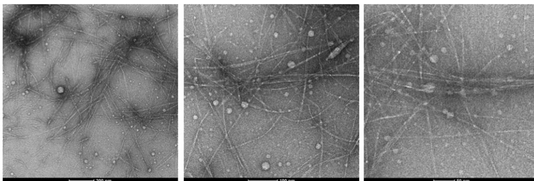
Figure S42. TEM image of photoactivated DBS-CONH<sub>2</sub>NH<sub>2</sub>/gellan gum hybrid gel prepared using CaCO<sub>3</sub> as a cross-linker and DPIN as a pH activator. Scale bars (from left to right): 200 nm, 100 nm and 50 nm.
