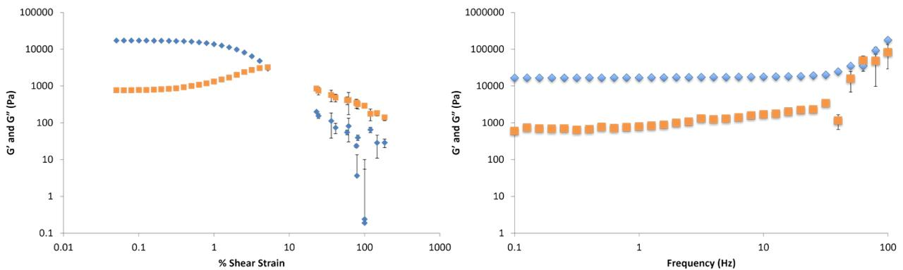
Figure S37. Elastic ( $G'$ , blue circles) and viscous ( $G''$ , red circles) moduli of DBS-CONHNH<sub>2</sub>/gellan gum hydrogel (0.3% wt/vol DBS-CONHNH<sub>2</sub> and 0.3% wt/vol gellan gum) prepared with 0.3% wt/vol CaCO<sub>3</sub> and 1.0% wt/vol GdL with increasing shear strain (left) and frequency (right).
