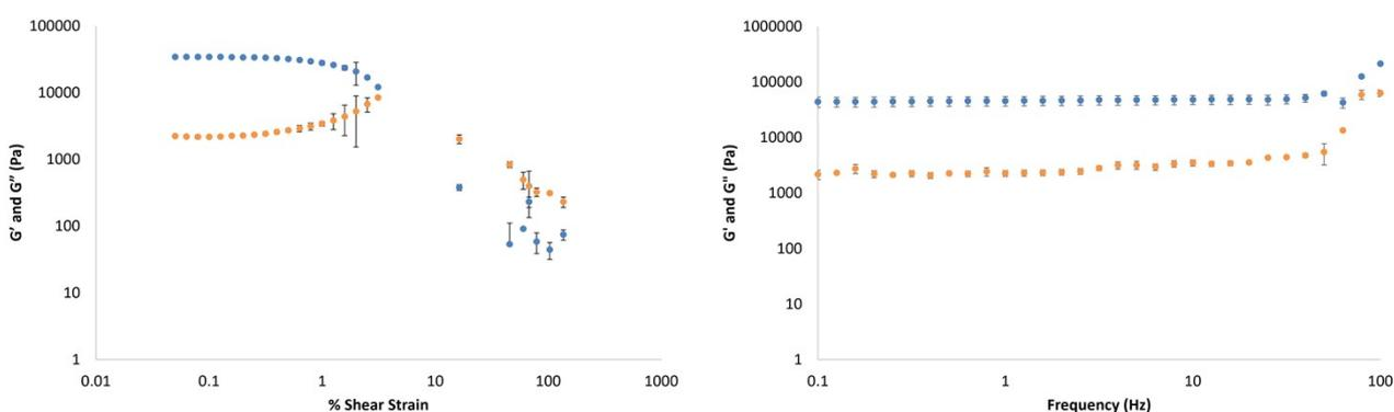
Figure S17. Elastic ( $G'$ , blue circles) and viscous ( $G''$ , orange circles) moduli of DBS-CONH<sub>2</sub>/gellan gum multicomponent hydrogel (0.3% wt/vol DBS-CONH<sub>2</sub> and 1.0% wt/vol gellan gum) with increasing shear strain (left) and frequency (right).
