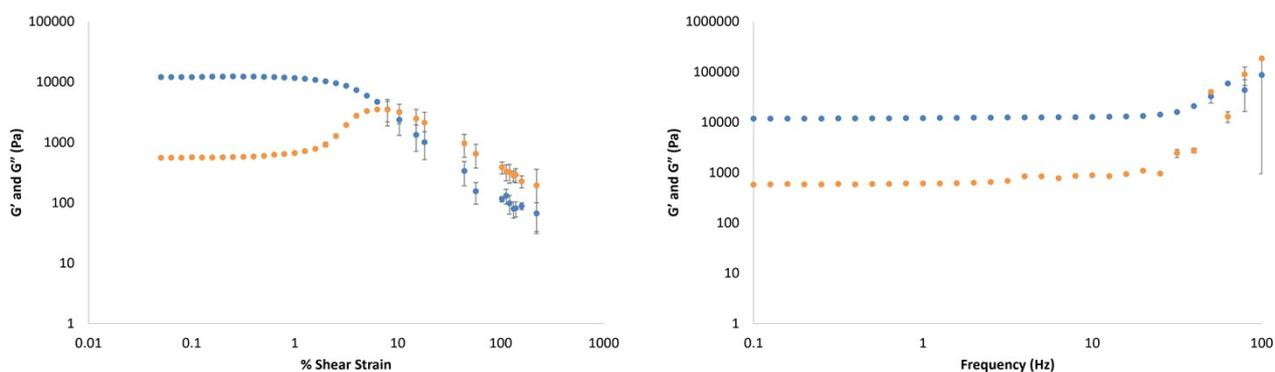
Figure S45. Elastic ( $G'$ , blue circles) and viscous ( $G''$ , red circles) moduli of photoactivated DBS-CONH<sub>2</sub>/gellan gum hydrogel (0.3% wt/vol DBS-CONH<sub>2</sub> and 0.3% wt/vol gellan gum) prepared with 0.15% wt/vol CaCO<sub>3</sub> and 0.8% wt/vol DPIN with increasing shear strain (left) and frequency (right).
