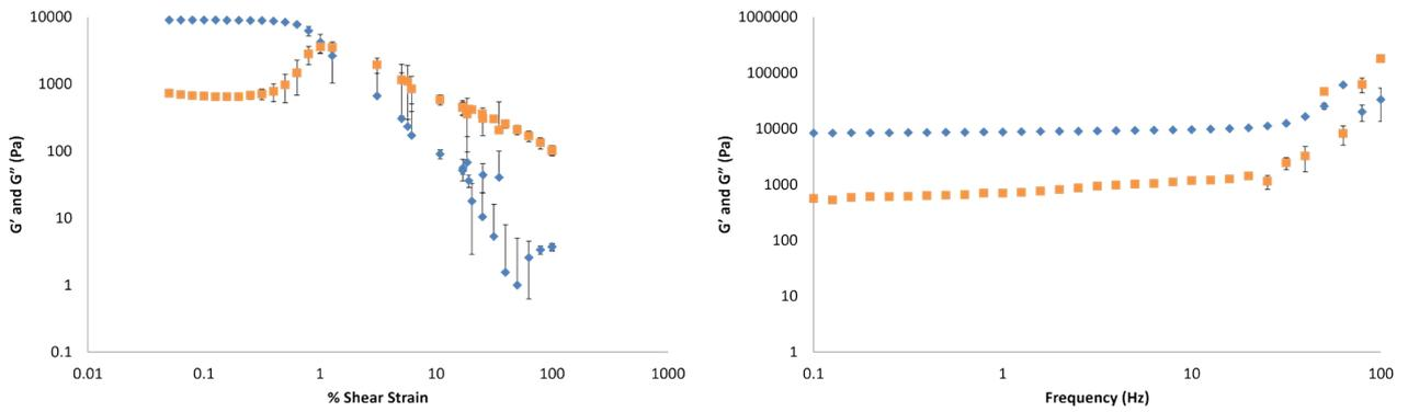
Figure S32. Elastic ( $G'$ , blue circles) and viscous ( $G''$ , red circles) moduli of gellan gum hydrogel (0.8% wt/vol) prepared with 0.15% wt/vol  $\text{CaCO}_3$  and 1.0% wt/vol GdL with increasing shear strain (left) and frequency (right).
