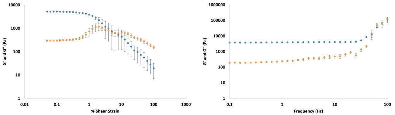
Figure S14. Elastic ( $G'$ , blue circles) and viscous ( $G''$ , orange circles) moduli of DBS-CONH<sub>2</sub>/gellan gum two-component hydrogel (0.3% wt/vol DBS-CONH<sub>2</sub> and 0.1% wt/vol gellan gum) with increasing shear strain (left) and frequency (right).
