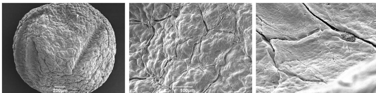
Figure S26. SEM images of DBS-CONHNH<sub>2</sub>/gellan gum whole gel bead and surface (prepared using CaCO<sub>3</sub> as a cross-linker and GdL as a pH activator). Scale bars (from left to right): 200 (left) and 100 μm (centre and right).
