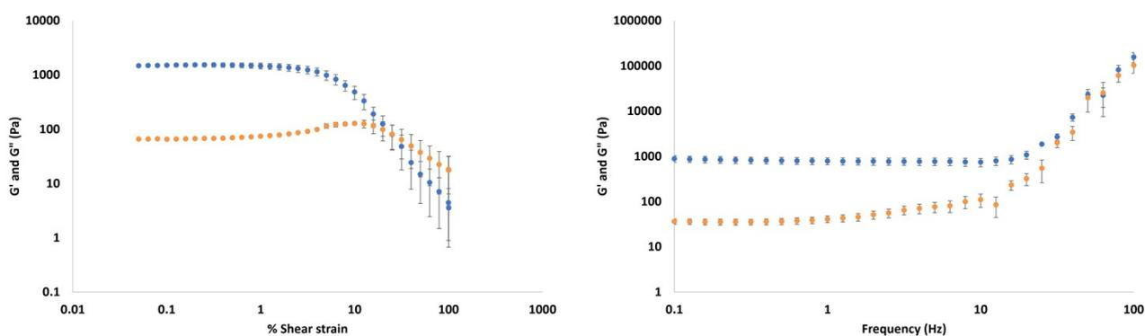
Figure S9. Elastic (G', blue circles) and viscous (G'', orange circles) moduli of DBS-CONH<sub>2</sub> hydrogel (0.4% wt/vol) with increasing shear strain (left) and frequency (right).
