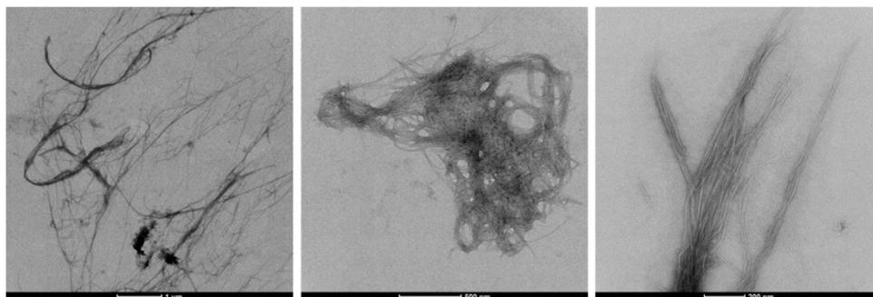
Figure S6. TEM images of gellan gum gel cross-linked with  $\text{CaCl}_2$ . Scale bars (from left to right): 1  $\mu\text{m}$  (left), 200 nm (centre) and 100 nm (right).
