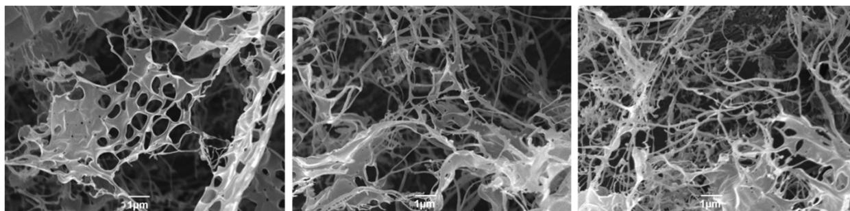
Figure S28. SEM images of DBS-CONHNNH<sub>2</sub>/gellan gum hybrid gel prepared in sample vials using CaCO<sub>3</sub> as a cross-linker and GdL as a pH activator. Scale bars: 1 μm.
