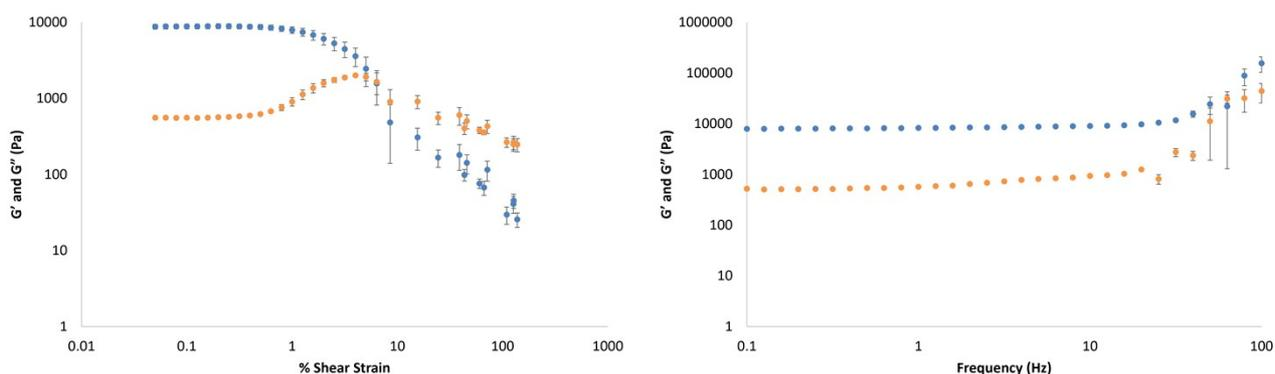
Figure S46. Elastic ( $G'$ , blue circles) and viscous ( $G''$ , red circles) moduli of photoactivated gellan gum hydrogel (0.6% wt/vol) prepared with 0.15% wt/vol CaCO<sub>3</sub> and 0.8% wt/vol DPIN with increasing shear strain (left) and frequency (right).
