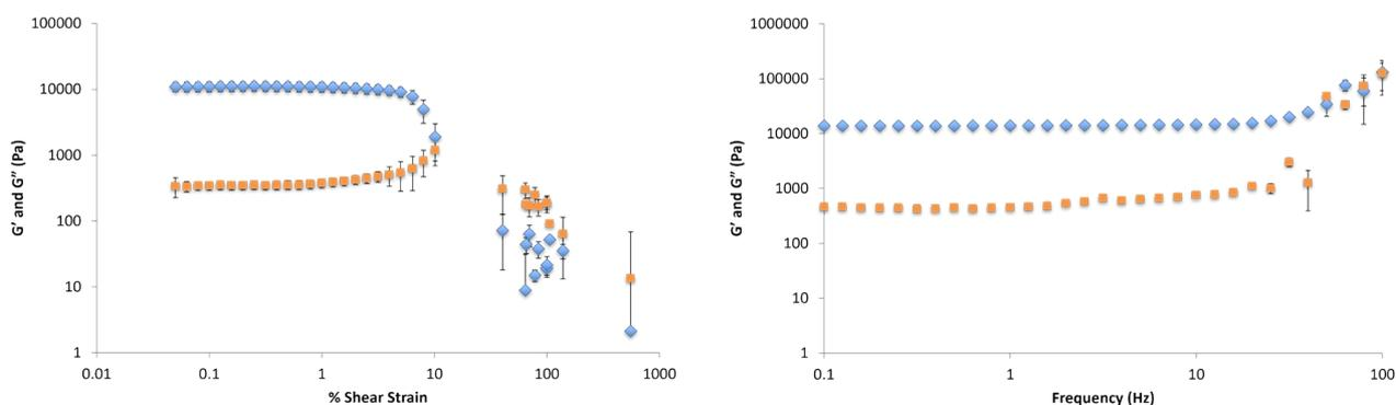
Figure S39. Elastic ( $G'$ , blue circles) and viscous ( $G''$ , red circles) moduli of DBS-CONH<sub>2</sub>/gellan gum hydrogel (0.3% wt/vol DBS-CONH<sub>2</sub> and 0.3% wt/vol gellan gum) prepared with 0.15% wt/vol CaCO<sub>3</sub> and 1.2% wt/vol GdL with increasing shear strain (left) and frequency (right).
