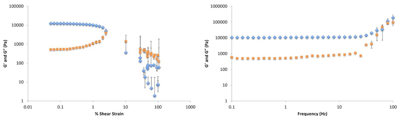
Figure S38. Elastic ( $G'$ , blue circles) and viscous ( $G''$ , red circles) moduli of DBS-CONH<sub>2</sub>/gellan gum hydrogel (0.3% wt/vol DBS-CONH<sub>2</sub> and 0.3% wt/vol gellan gum) prepared with 0.15% wt/vol CaCO<sub>3</sub> and 0.8% wt/vol GdL with increasing shear strain (left) and frequency (right).
