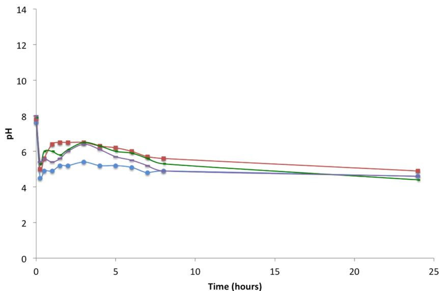
Figure S19. pH changes over time during the formation of gellan gum gels ( $\text{CaCO}_3$  - 0.15% wt/vol and GdL - 0.8% wt/vol) prepared using a gellan gum concentration of 0.4% wt/vol (blue line), 0.6% wt/vol (red line), 0.8% wt/vol (green line) or 1.3% wt/vol (purple line).
