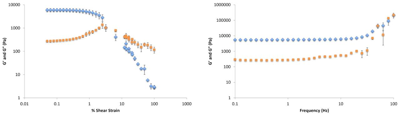
Figure S36. Elastic ( $G'$ , blue circles) and viscous ( $G''$ , red circles) moduli of DBS-CONHNH<sub>2</sub>/gellan gum hydrogel (0.3% wt/vol DBS-CONHNH<sub>2</sub> and 0.3% wt/vol gellan gum) prepared with 0.0075% wt/vol CaCO<sub>3</sub> and 1.0% wt/vol GdL with increasing shear strain (left) and frequency (right).
