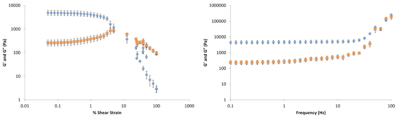
Figure S54. Elastic ( $G'$ , blue circles) and viscous ( $G''$ , red circles) moduli of DBS-CONH<sub>2</sub>/gellan gum hydrogel (0.3% wt/vol DBS-CONH<sub>2</sub> and 0.3% wt/vol gellan gum – loaded with 3 mL AgNO<sub>3</sub> 10 mM) with increasing shear strain (left) and frequency (right).
