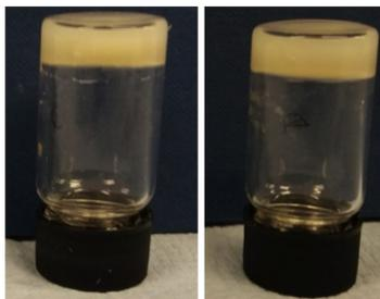
Figure S40. Photographic images of DBS- $\text{CONHNH}_2$ /gellan gum (left) and gellan gum gels (right) prepared by photo-activation using  $\text{CaCO}_3$  (0.15% wt/vol) and DPIN (0.8% wt/vol).
