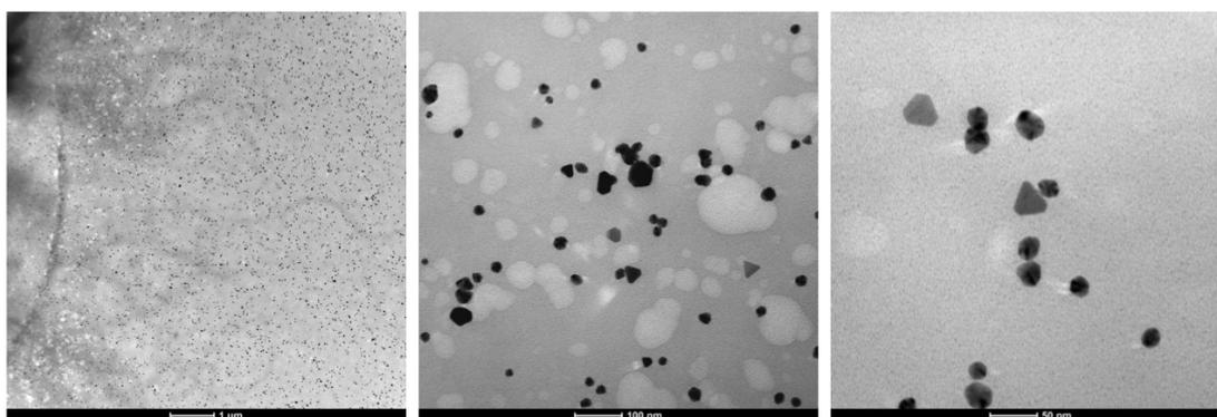
Figure S49. TEM images of DBS-CONH<sub>2</sub>/gellan gum gel beads incorporating AgNPs. Scale bars (from left to right): 1 μm, 100 nm and 50 nm.
