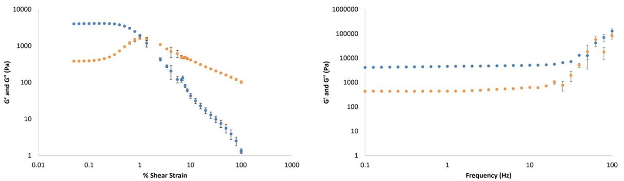
Figure S11. Elastic ( $G'$ , blue circles) and viscous ( $G''$ , orange circles) moduli of gellan gum hydrogel (0.6% wt/vol) with increasing shear strain (left) and frequency (right).
