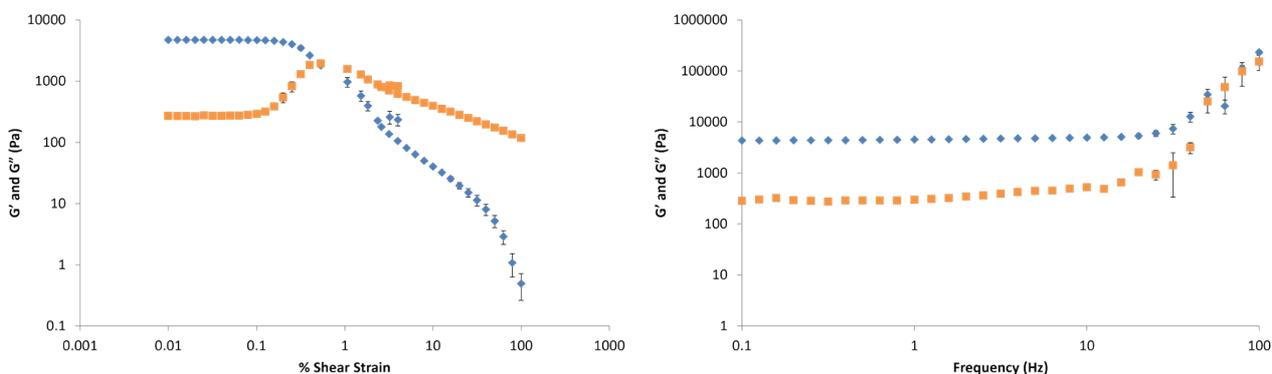
Figure S31. Elastic ( $G'$ , blue circles) and viscous ( $G''$ , red circles) moduli of gellan gum hydrogel (0.6% wt/vol) prepared with 0.15% wt/vol CaCO<sub>3</sub> and 1.0% wt/vol GdL with increasing shear strain (left) and frequency (right).
