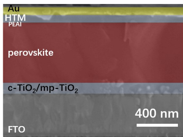
Figure S4. Cross-sectional SEM image of a typical PSC (the concentration of HTM is 40 mg mL -1 ).
