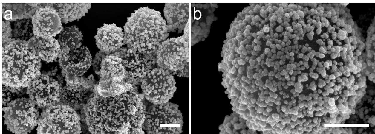
**Figure S11.** SEM micrographs of **C $\mu$ P-AuNP-2** composite particles. Scale bars show **(a)** 500 nm; and **(b)** 500 nm.
