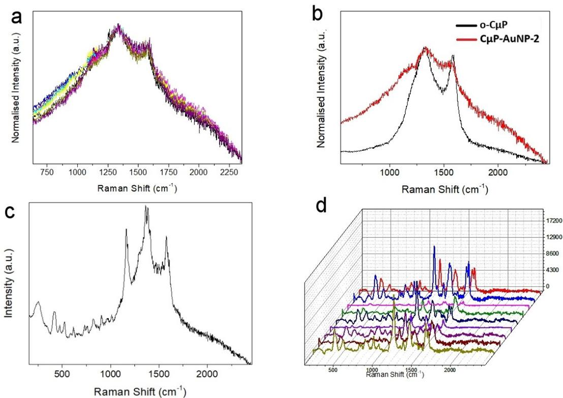
**Figure S19** (a) Normalized Raman spectra for eight  $C\mu P-AuNP-2$  particles. (b) Averaged normalized Raman spectra of  $C\mu P-AuNP-2$  particles (black trace)  $o-C\mu P$  particles (red trace). (c) Raman spectrum from trapped  $C\mu P-AuNP-2$  composite particle incubated with  $10 \mu M$  MG. (d) Raman spectrum  $C\mu P-AuNP-2$  composite particles incubated with  $10 \mu M$  MG. Each trace shows an individual particle. Spectra recorded in  $H_2O$  with 785 nm excitation.
