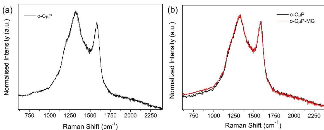
**Figure S13.** Normalized Raman spectra for (a) an optically trapped **o-C<sub>μ</sub>P** particle recorded in H<sub>2</sub>O with 785 nm excitation. (b) Comparison recorded for **o-C<sub>μ</sub>P** incubated in the presence of 10 μM MG.
