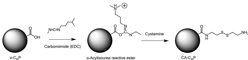
**Scheme S1.** Reaction scheme for the preparation of cystamine functionalized **CA-C $\mu$ P**.
