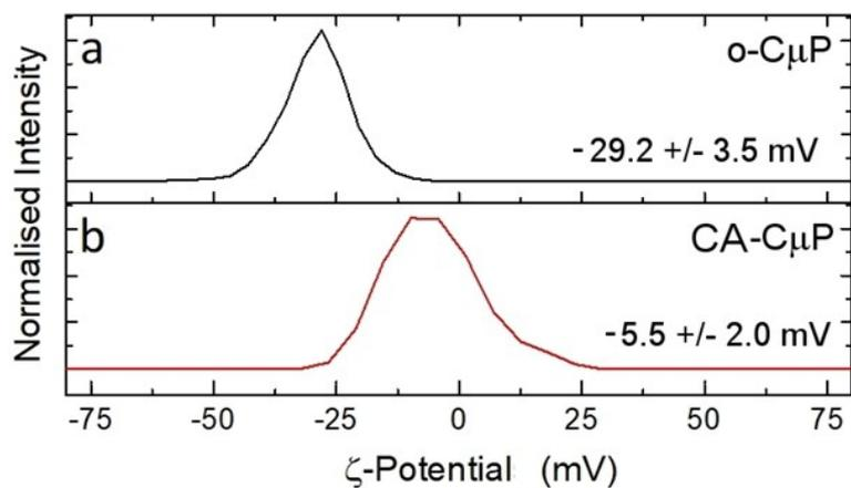
**Figure S3:** ζ-potential measurements of (a) **o-CμP** and (b) **CA-CμP** recorded in 10 mM NaCl at pH 7.
