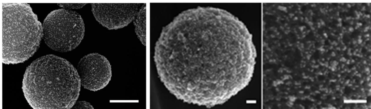
**Figure S6.** Additional representative SEM micrographs of C $\mu$ P-AuNP(DMAP) composites. Scale bars shows (a) 500 nm (b-c) 100 nm.
