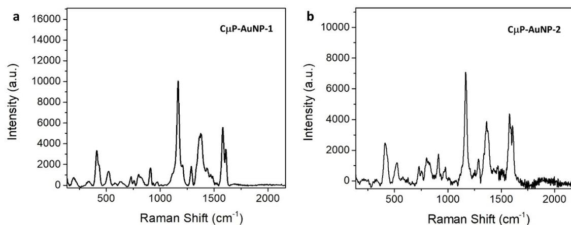
**Figure S20.** Averaged Raman spectra of (a)  $C\mu P-AuNP-1$  and (b)  $C\mu P-AuNP-2$  recorded for particles incubated with  $10 \mu M$  MG. Spectra recorded in  $H_2O$  with 785 nm excitation.
