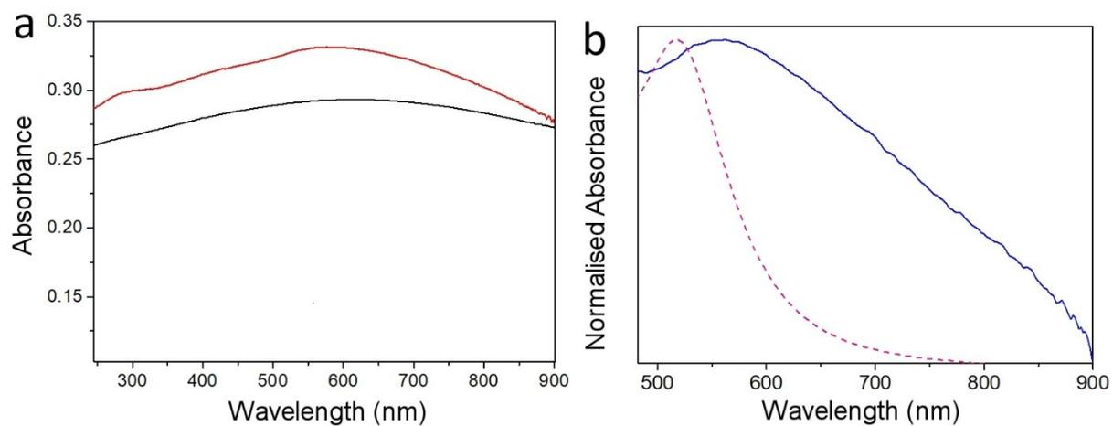
**Figure S7** UV-Vis spectra of (a) o-CμP (black trace) and CμP-AuNP(DMAP) (red trace); and (b) AuNP(DMAP) (red trace) and difference spectrum (blue trace). Spectra recorded in ddiH<sub>2</sub>O in a quartz cuvette.
