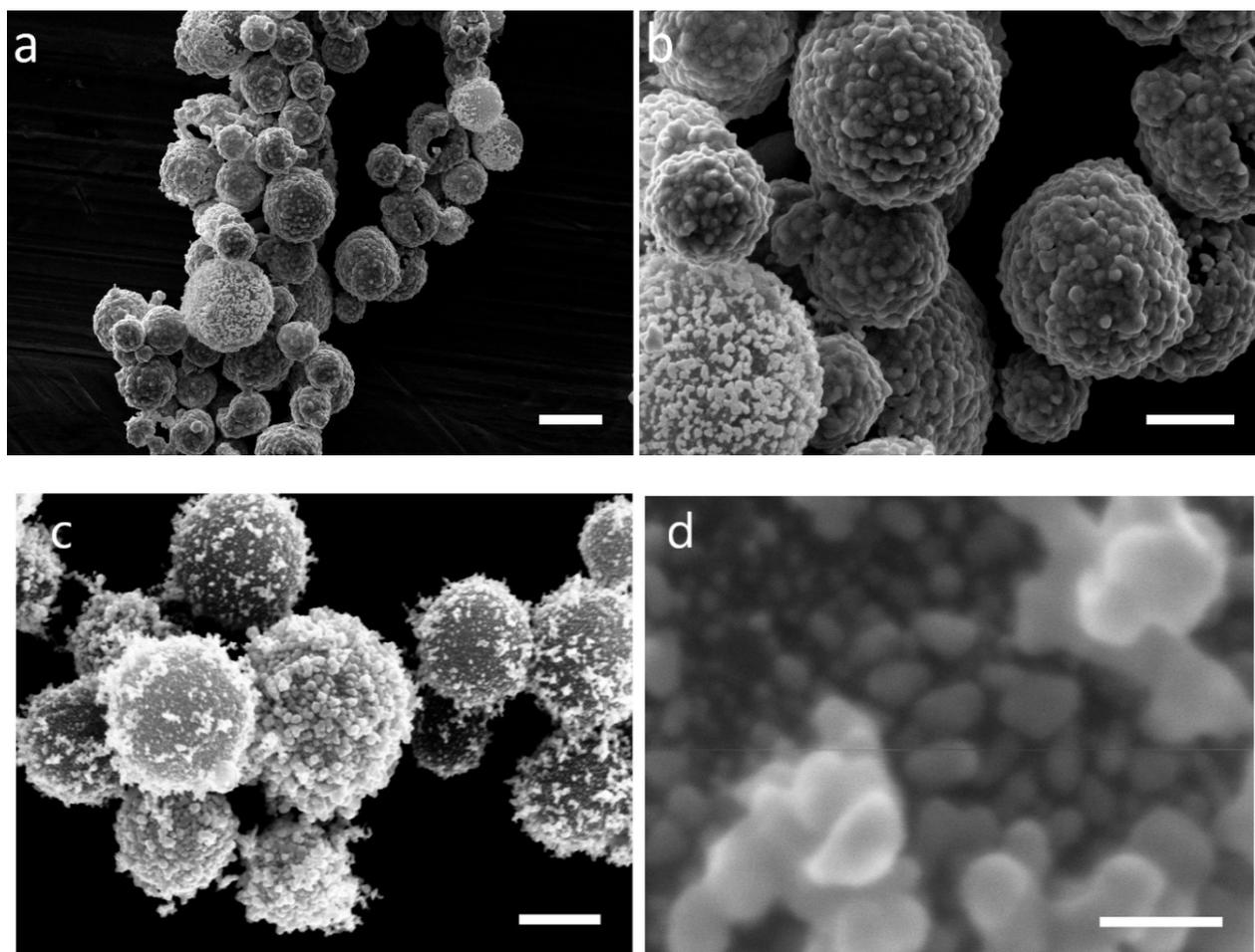
**Figure S9.** SEM micrographs of Hydroquinone/ $\text{HAuCl}_4$  treated  $\text{C}\mu\text{P-AuNP(DMAP)}$  composite particles  $\text{C}\mu\text{P-AuNP-1}$ . Scale bars show; (a) 1  $\mu\text{m}$ ; (b, c) 500 nm and (d) 50 nm.
