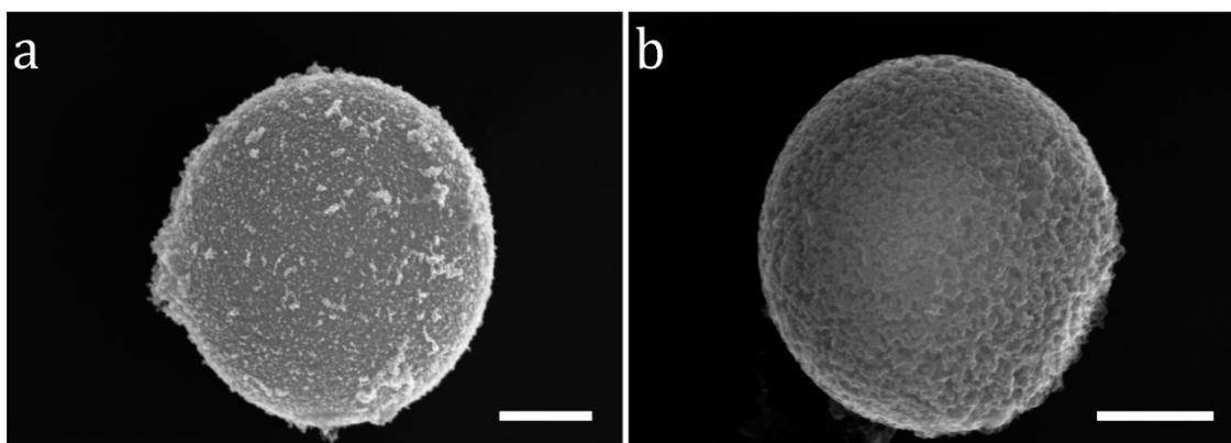
**Figure S8.** CμP-AuNP(DMAP) (a) before; and (b) after; gold digestion by sonication in 5 % aqua regia solution. Scale bars show 500 nm.
