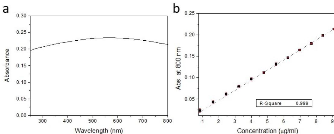
**Figure S1:** (a) Absorbance spectrum of an aqueous dispersion of C $\mu$ P; and (b) Linear fit of absorption at 800 nm vs. concentration of C $\mu$ P (error bars show standard deviation from three measurements). Spectra recorded in ddiH $_2$ O at rt.
