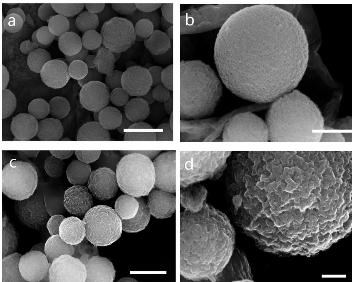
**Figure S2:** SEM micrographs of (a-b) o-C $\mu$ P formed by reacting in 5 M HNO $_3$  at 80  $^{\circ}$ C for 2 h. Scale bars are 1  $\mu$ m (RHS) and 500 nm (LHS) respectively. (c-d) CA-C $\mu$ P. Scale bars show (c) 1  $\mu$ m and (d) 200 nm.
