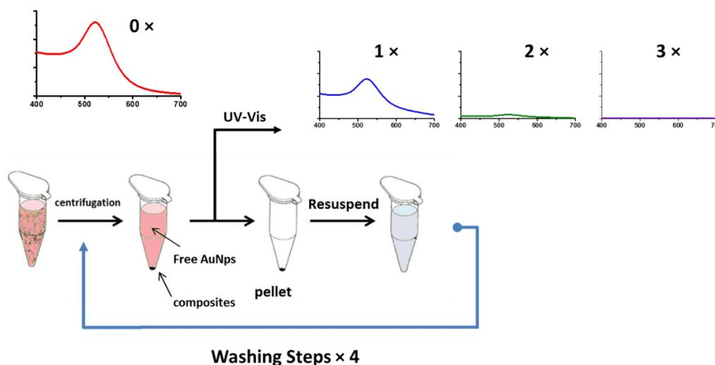
**Scheme S2.** Schematic of centrifugation washing showing visible absorption spectra of the supernatant of composite solutions following successive washing steps and SEM micrograph of composites following four washing steps.
