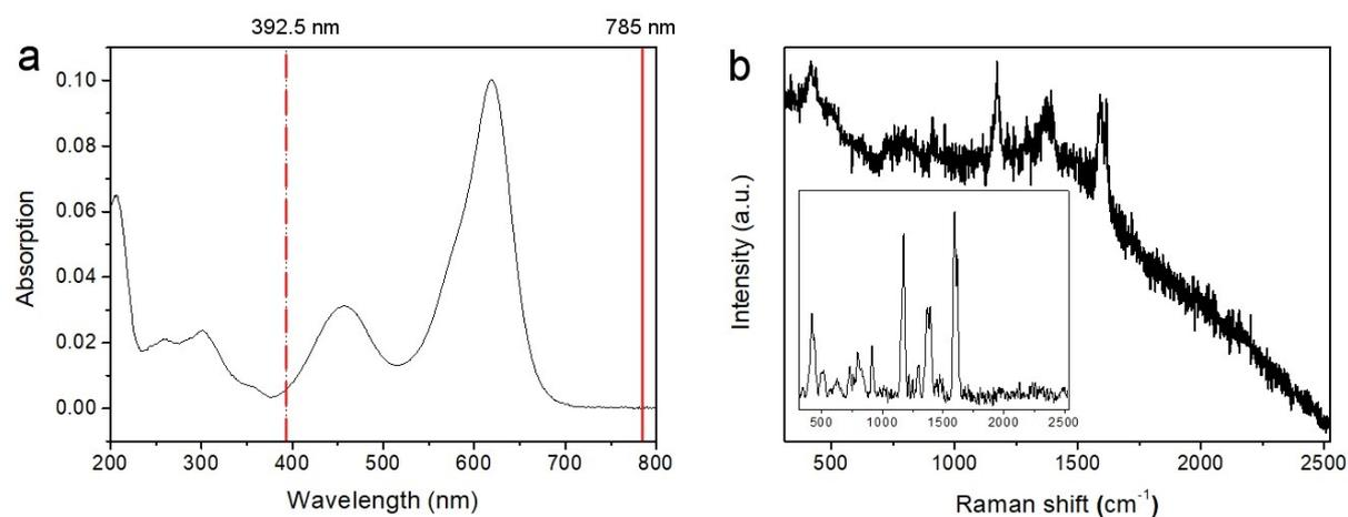
**Figure S12.** **(a)** UV-Vis absorption spectrum of malachite green isothiocyanate. Solid line shows laser excitation wavelength, dashed line shows the two photon wavelength of this laser. (Recorded in diH<sub>2</sub>O). **(b)** Raman spectrum of solid film of malachite green drop cast from 1 mM MG solution in ethanol with 785 nm excitation. Insert shows spectrum following smoothing and baseline correction.
