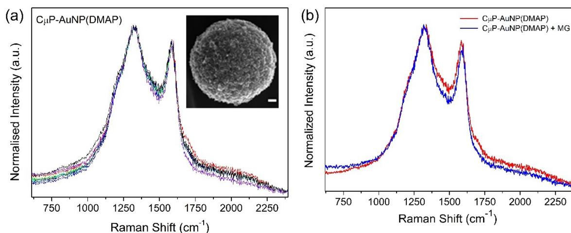
**Figure S14.** Normalized Raman spectra for (a) **C<sub>μ</sub>P-AuNP(DMAP)** composite particles, inset showing the SEM image with a scale bar of 100 nm, and (b) **C<sub>μ</sub>P-AuNP(DMAP)** incubated with 10 μM MG recorded in H<sub>2</sub>O with 785 nm excitation.
