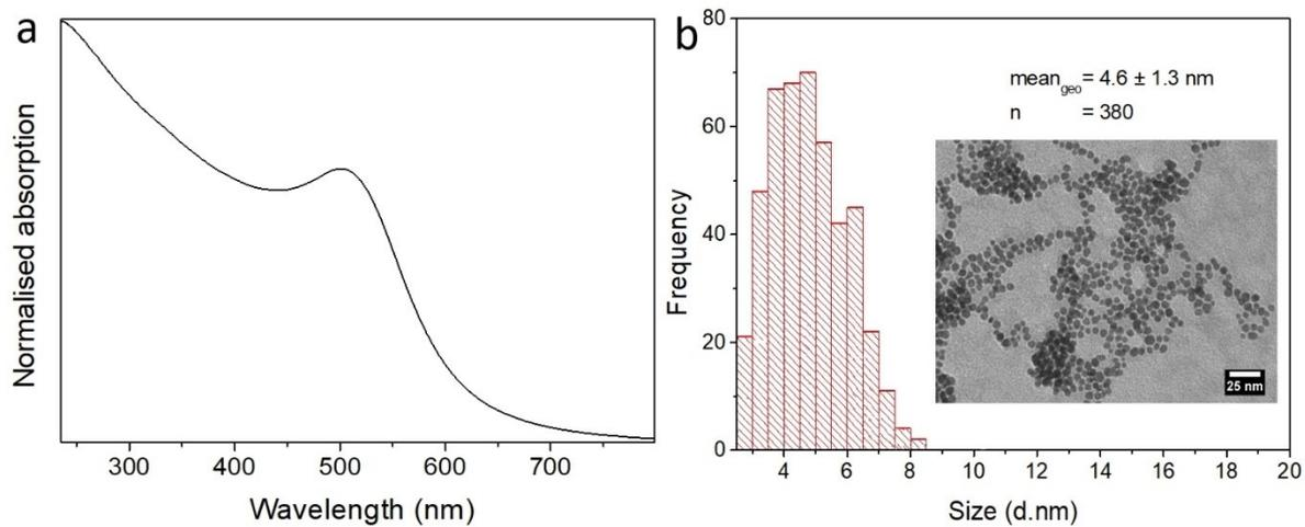
**Figure S5.** (a) Normalised absorption spectrum of AuNP(BH) in ddiH<sub>2</sub>O. (b) TEM micrograph size distribution analysis of AuNP(BH). Insert is a TEM micrograph of these nanoparticles.
