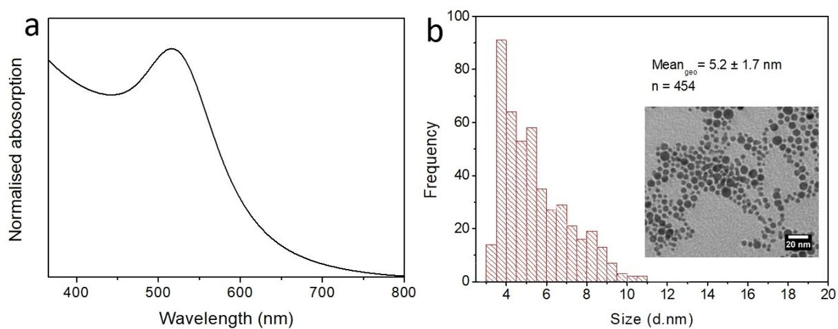
**Figure S4:** (a) Normalized absorption spectrum of AuNP(DMAP) in ddiH<sub>2</sub>O. (b) TEM micrograph size distribution analysis of AuNP(DMAP) nanoparticle. Insert: TEM micrograph of these nanoparticles.
