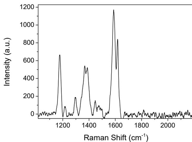
**Figure S18.** Bulk solid Raman spectrum from 10  $\mu$ M MG-incubated **C $\mu$ P-AuNP-1** particles. Spectra recorded with 514 nm excitation from a sample drop cast on CaF<sub>2</sub>.
