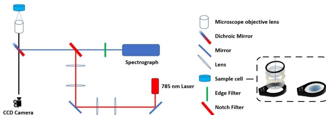
**Scheme S3.** Schematic representation of set-up for single particle Raman measurements
