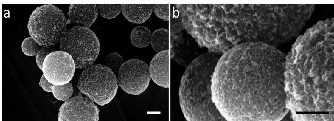
**Figure S10.** Additional representative SEM micrographs of  $\text{C}\mu\text{P-AuNP(BH)}$  composites. (Scale bars show; (a) 500 nm; and (b) 200 nm).
