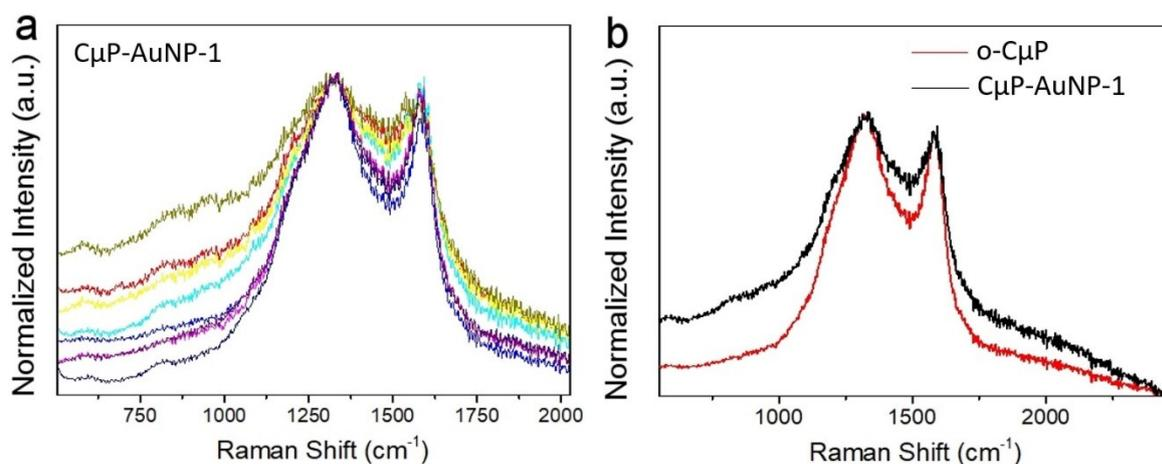
**Figure S16.** (a) Normalized Raman spectra for a selection of **C $\mu$ P-AuNP-1** particles, showing the variable dampening in carbon D and G bands. Each trace shows an individual particle. (b) Averaged normalized Raman spectra of **o-C $\mu$ P** particles (red trace) and **C $\mu$ P-AuNP-1** particles (black trace) Spectra recorded in H<sub>2</sub>O with 785 nm excitation.
