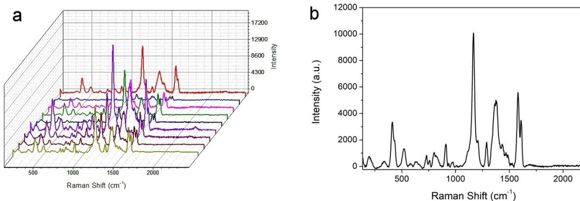
**Figure S17.** (a) Analyte Raman spectrum from **C $\mu$ P-AuNP-1** composite particles incubated with 10  $\mu$ M MG. Each trace shows an individual particle. (b) Average SERS spectrum from all measured particles.
