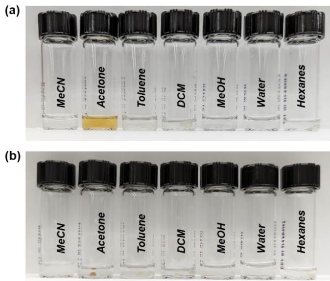
Figure S7. Images of (a) PEI and (b) PPI in liquid solvents after 7 days of storage at ambient temperature and pressure.
