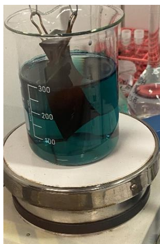
Fig.S2: Setup of the dip-coating of carbon paper via chemical oxidative polymerization of aniline.
