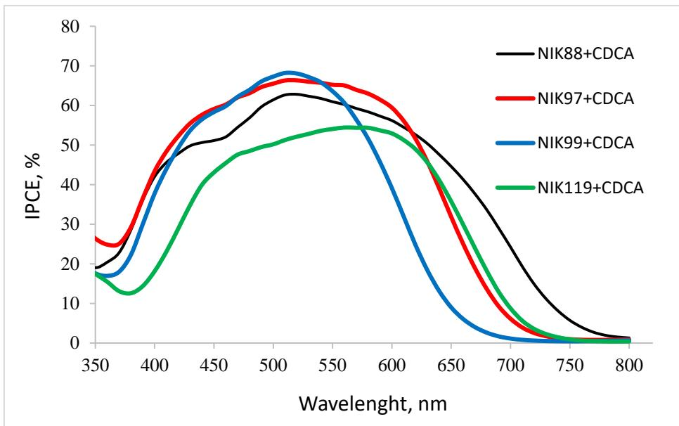
**Fig. S2.** The IPCE spectra for DSSCs based on the dyes **NIK** series with CDCA addition as co-adsorbent
