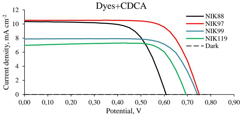
**Fig. S1.** The *J-V* curves for DSSCs based on the dyes **NIK** series with CDCA addition as co-adsorbent
