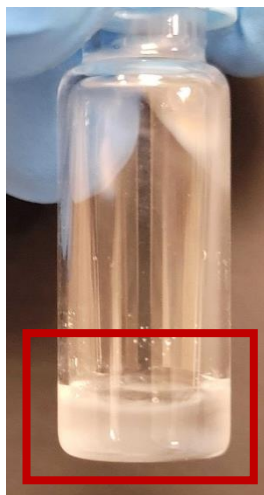
Figure S22: Sample composed of the 80 mol% Choline Chloride with Acetamide. The sample was heated using a hotplate and formed an opaque solution, which is a sign of formation of two phases.
