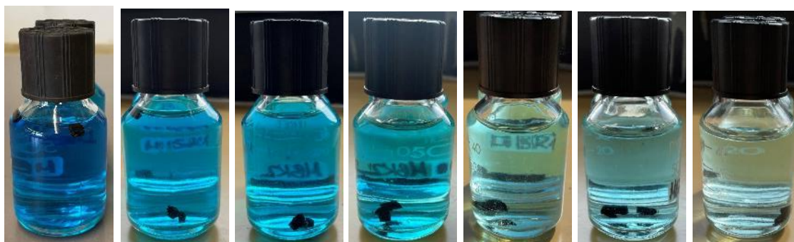
Fig. S15 MB adsorption kinetics of MIL-53(Al)@Pine-MA (50 ml MB solution with 5 mg L -1 ). From left to right: start, 1 h, 2 h, 8 h, 24 h, 32 h, 48 h.
