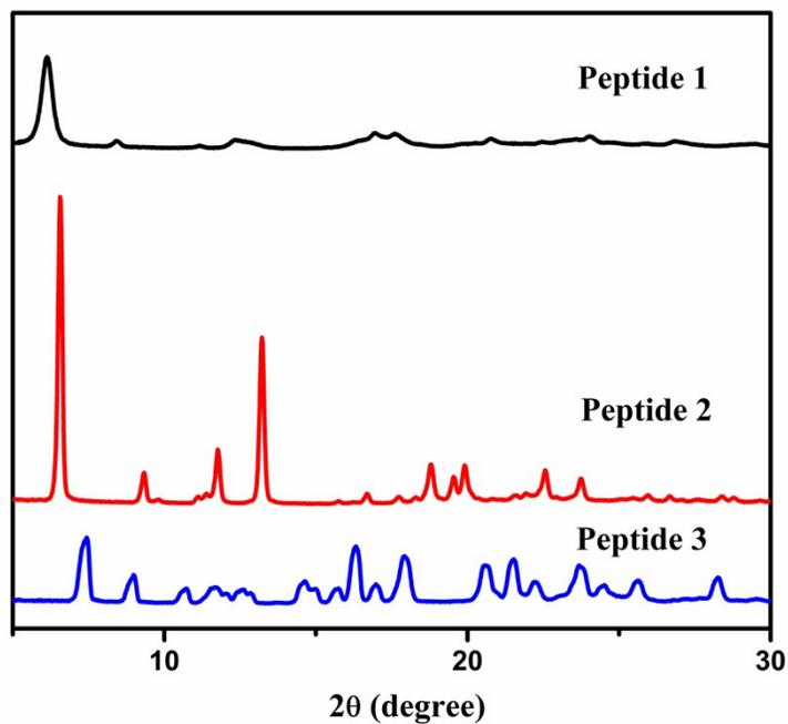
**Fig. S3.** WAXS spectra of peptides 1-3. ). Peptides 2 and 3 polydisperse microspheres show sharp reflections in the 5–25°  $2\theta$  range whereas only a very broad feature was observed for peptide 1 fibers.
