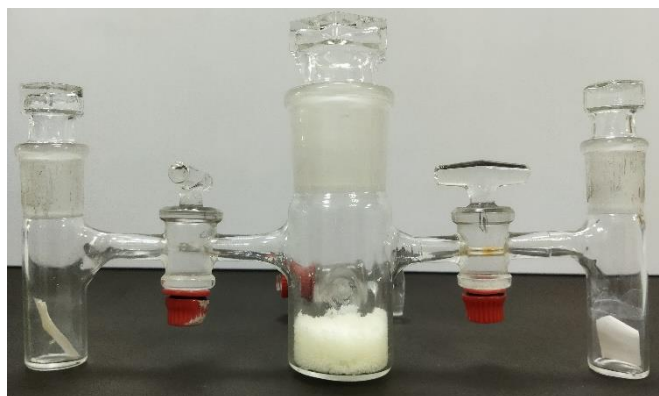
Figure S45: Digital image of set-up for demonstration of NO vapour detection by PABA@MOF-808@PVDF MMM.
