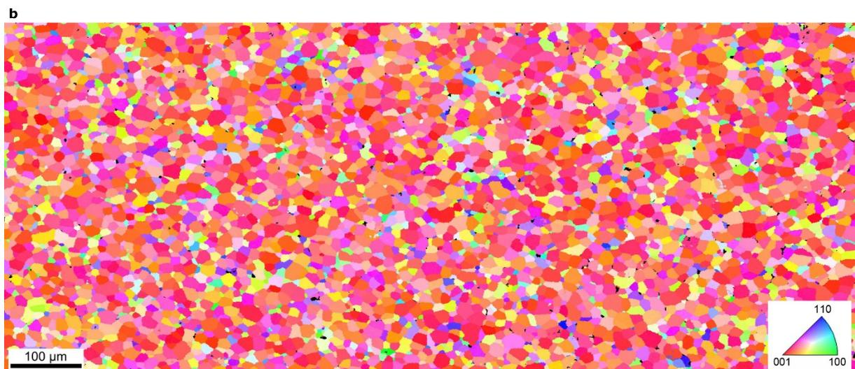
**Fig. S4.** Evidence for texture in the surface layer sintered with a single flash from a Xe-flash lamp. (a) Pole figure plot visualizing the crystallographic texture. (b) Inverse pole figure map of the underlying EBSD scan of a  $\text{TiO}_2$  sample. The texture analysis reveals a pronounced crystallographic texture with  $\langle 001 \rangle \parallel$  surface normal.
