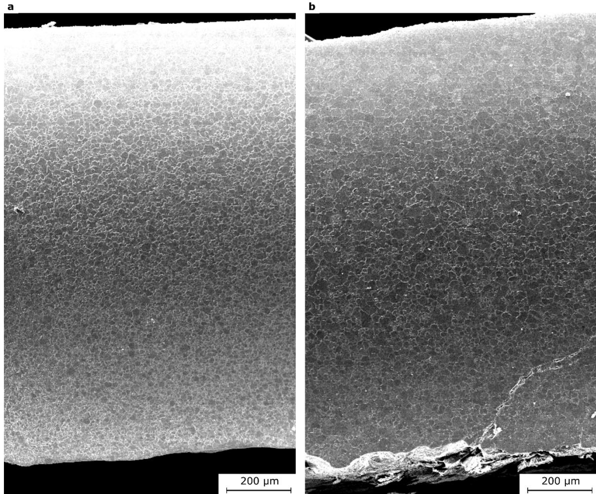
**Fig. S3.** Thermally etched cross section of TiO<sub>2</sub> samples equivalent to Fig. 1k+l. (a) Sintered with multi-pulse Xe-flash lamp. (b) Sintered with 450 nm laser.
