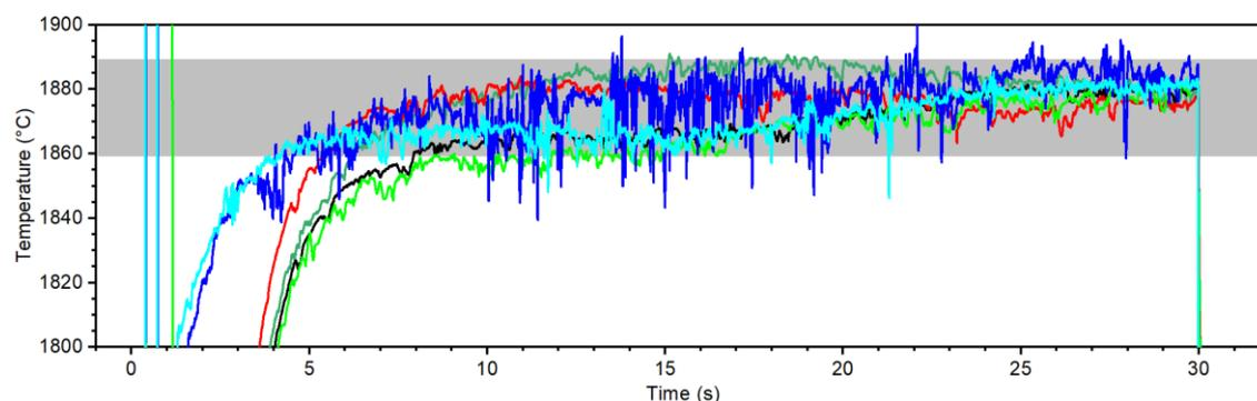
**Fig. S1:** Self-stabilization of temperature. Six recorded temperature curves from identical sintering experiments of SrTiO<sub>3</sub> with 170 Wcm<sup>-2</sup> of 450 nm laser light on expandable graphite. The light intensity rose from 0 % to 100 % within ≈1 ms and held for 30 seconds while the temperature was recorded with a pyrometer. An interval of ±15 K is highlighted in grey.
