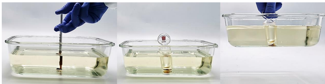
Figure S77. Underwater adhesion test of poly(TA-A) 8/1 .
