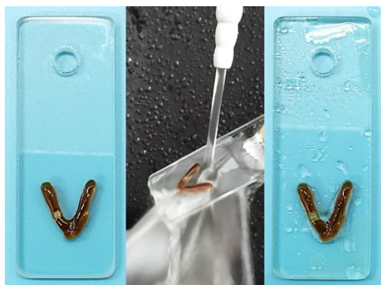
Figure S78. Water blasting (2 bar, 10 min) test of poly(TA-A) 8/1 .
