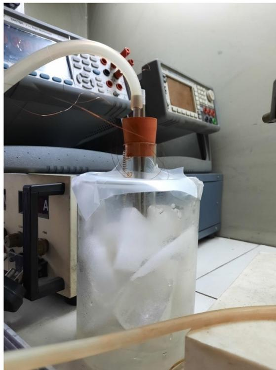
Figure S3: Low temperature enclosure for where the sensor has been placed.
