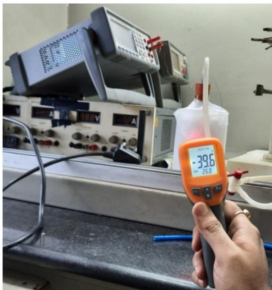
Figure S4: Temperature detection during cooling of sensor enclosure.
