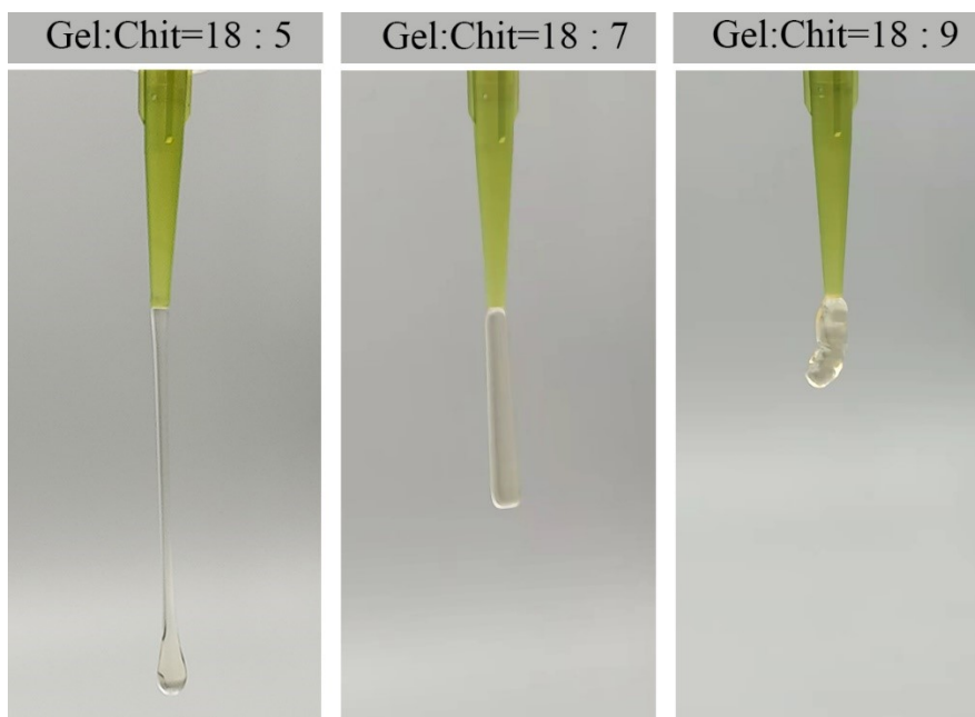
Figure S1. Optimization of Gel/Chit weight ratio by the printability of Gel/Chit-H + solution. The weight of chitosan was 5, 7, 9 g respectively (the total weight of chitosan and acetic acid solution is fixed at 100 g), and the weight of gelatin was fixed at 18 g.
