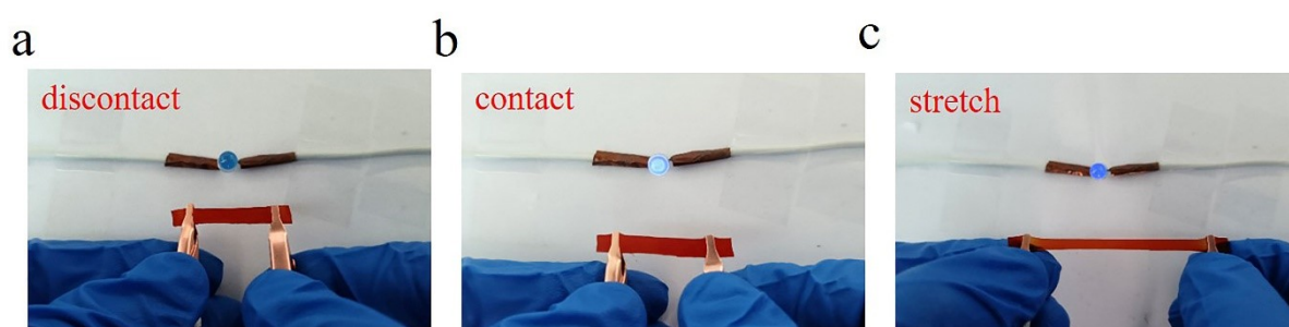
Fig. S12 Photographs of changes in LED brightness under (a) disconnect, (b) contact, and (c) stretch state.
