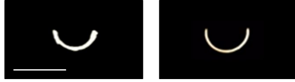
Fig. S14. The bending sample was made via the replica casting method with resin with 58 wt% alumina particles (Left). The bending sample with (\beta_1 - \beta_2) = 0.08 was made via the self-shaped printing method (Right). Scale bar indicates 7 mm.
