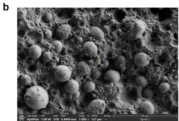
**Fig. S5** SEM images. (a). Fillers, (b) Polyurethane elastomer composite.
