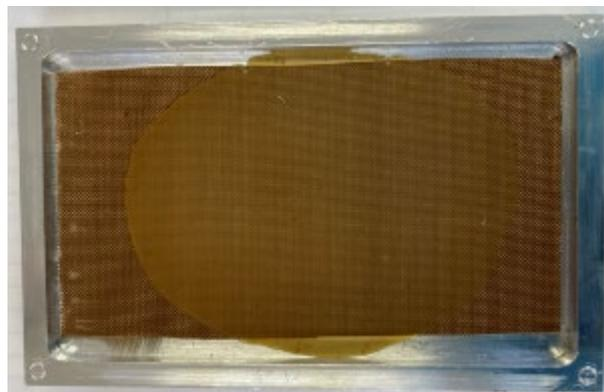
*Close up of the aluminium vessel, lined in PTFE, in which D series materials undergo mechanical recycling*
